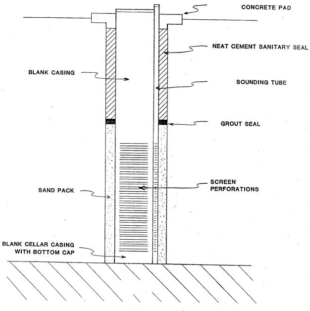
NOTE: ALL NEW WELLS WITHIN THE MONTEREY PENINSULA WATER MANAGEMENT DISTRICT MUST BE EQUIPPED WITH A SOUNDING TUBE. THE SKETCH SHOWN ABOVE ILLUSTRATES AN ACCEPTABLE METHOD FOR INSTALLING A SOUNDING TUBE.
