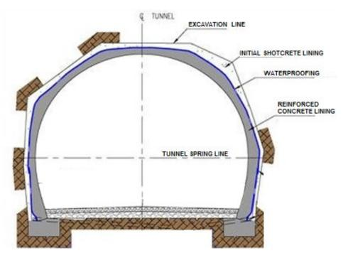
Figure 4-14 Concrete Tunnel Lining Schematic
