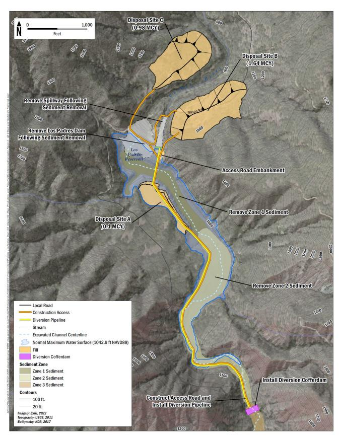
Figure 5-1 Overview of Alternative 2 (Dam and Sediment Removal)
