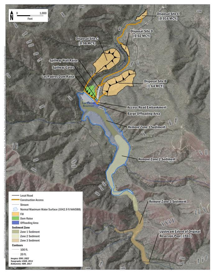
Figure 5-10 Overview of Alternative 3 (Storage Expansion and Dredging)
