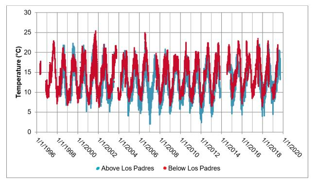
Figure 2-29 Carmel River Water Temperature above and below Los Padres Reservoir
