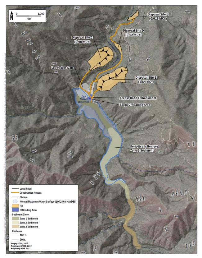
Figure 4-6 Alternative 4 (Recover Storage Capacity with Excavation)
