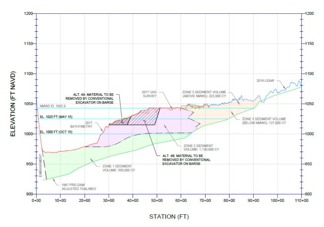
Figure 4-7 Material Dredging by Equipment Type and Water Level
