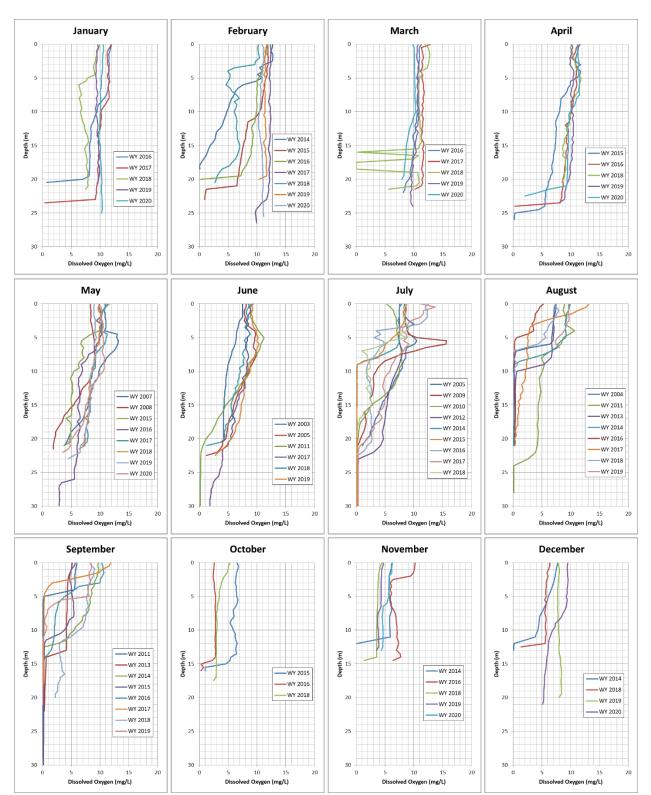
Figure 2-27 Los Padres Reservoir Dissolved Oxygen Profiles
