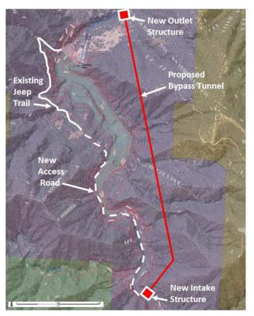
Figure 4-4 Bypass Tunnel Location
