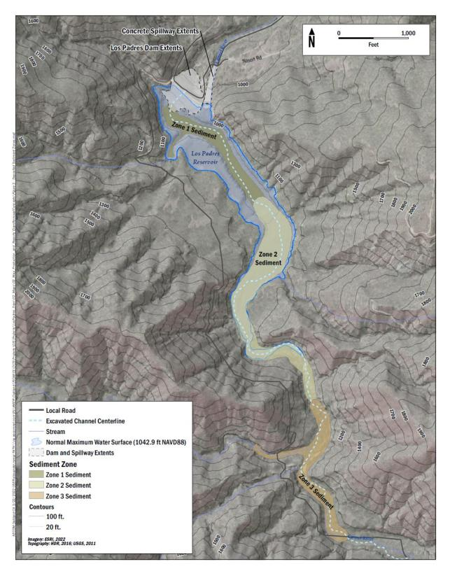
Figure 2-17 Plan View of Accumulated Sediment Zones
