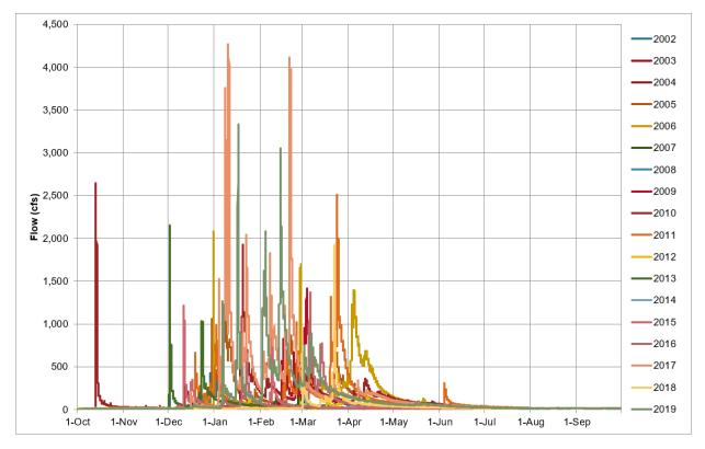
Figure 2-25 Carmel River Flows at the MPWMD Gauge Below Los Padres Dam (Water Years 2002 – 2019)
