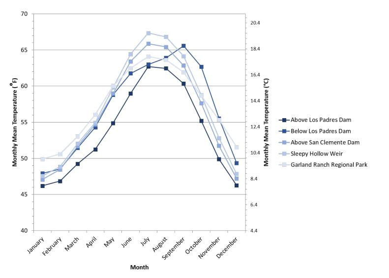
Figure 2-30 Average of Daily Carmel River Water Temperature for a Given Month before San Clemente Dam Removal (January 1996 through May 2014)
