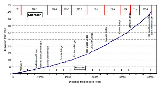
Figure 2-38 Longitudinal Profile of the Carmel River
