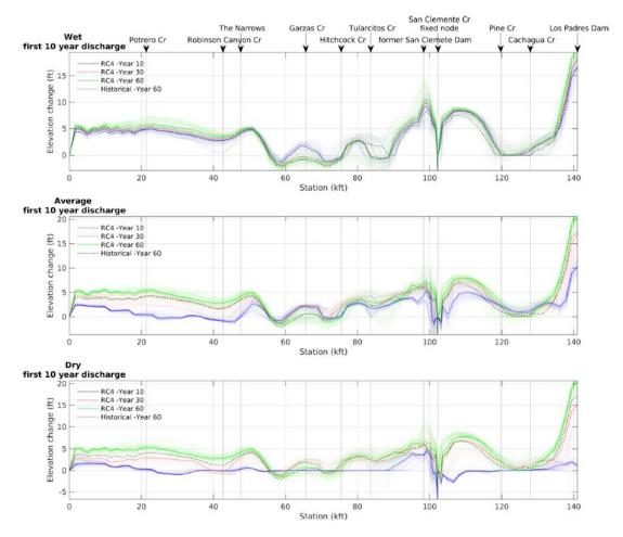
Figure 4-16 Change in Elevation Compared to the Initial Elevation Profile from 2017 for the Pulsed Supply Simulation
