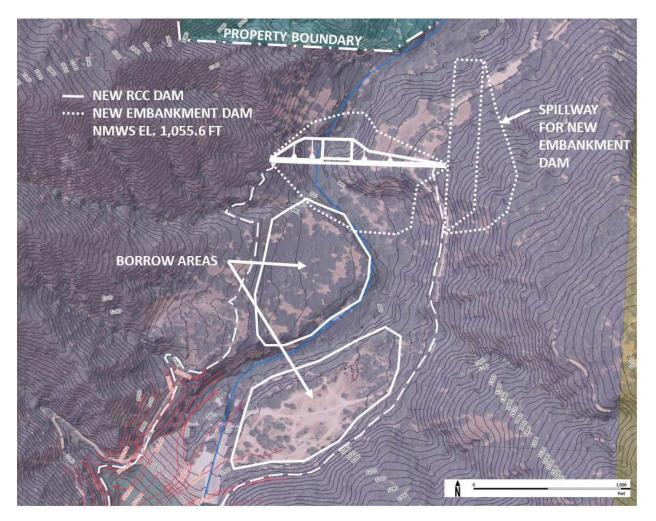
Figure 4-3 New Downstream Dam Concept Plan
