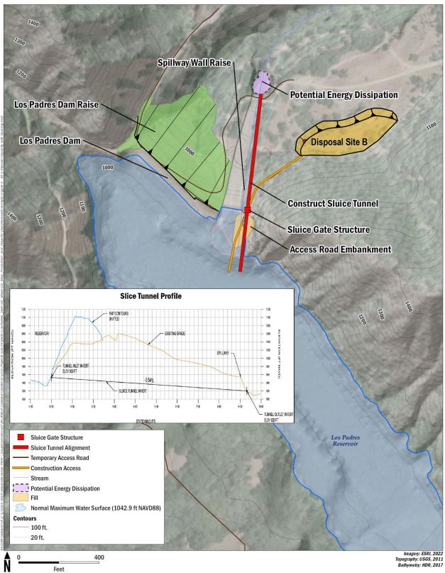
Figure 4-10 Overview of Alternative 5 (Recover Storage Capacity with Sluice Tunnel)
