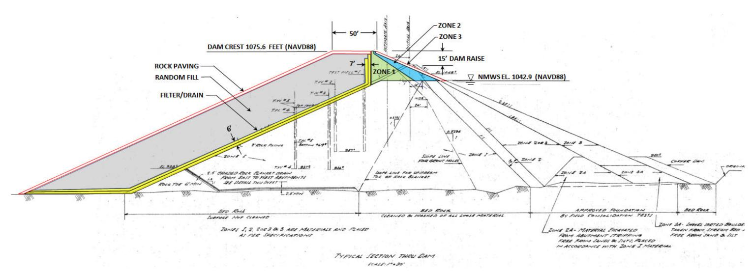
Figure 5-18 Dam Raise Schematic
