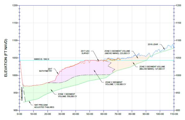
Figure 2-18 Profile View of Accumulated Sediment Zones
