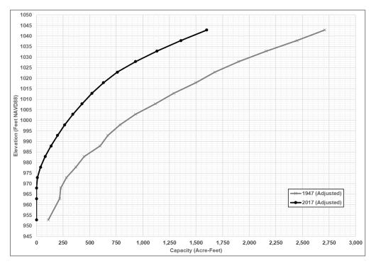
Figure 2-13 Los Padres Reservoir Stage-Storage Curve
