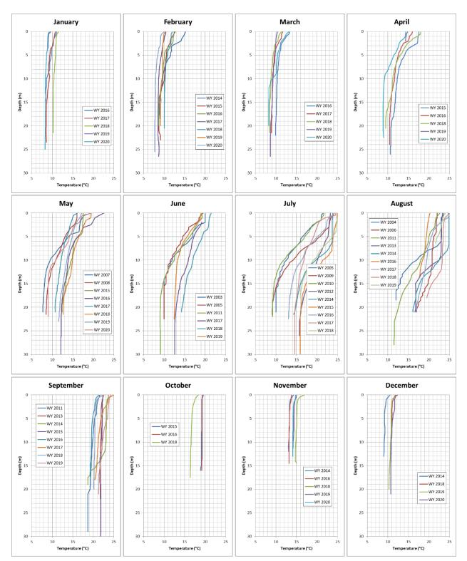
Figure 2-26 Los Padres Reservoir Water Temperature Profiles
