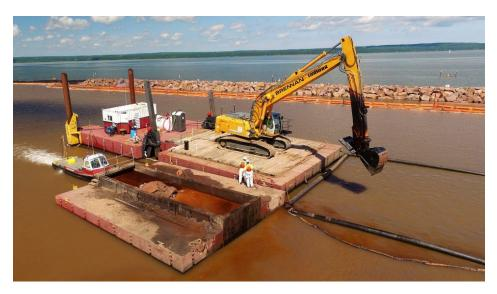
Figure 5-20 Conventional Excavator on Flexi-Float Barge
