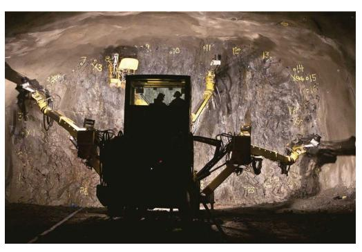
Figure 4-13 Self-Drilling Multiple Boom Jumbo
