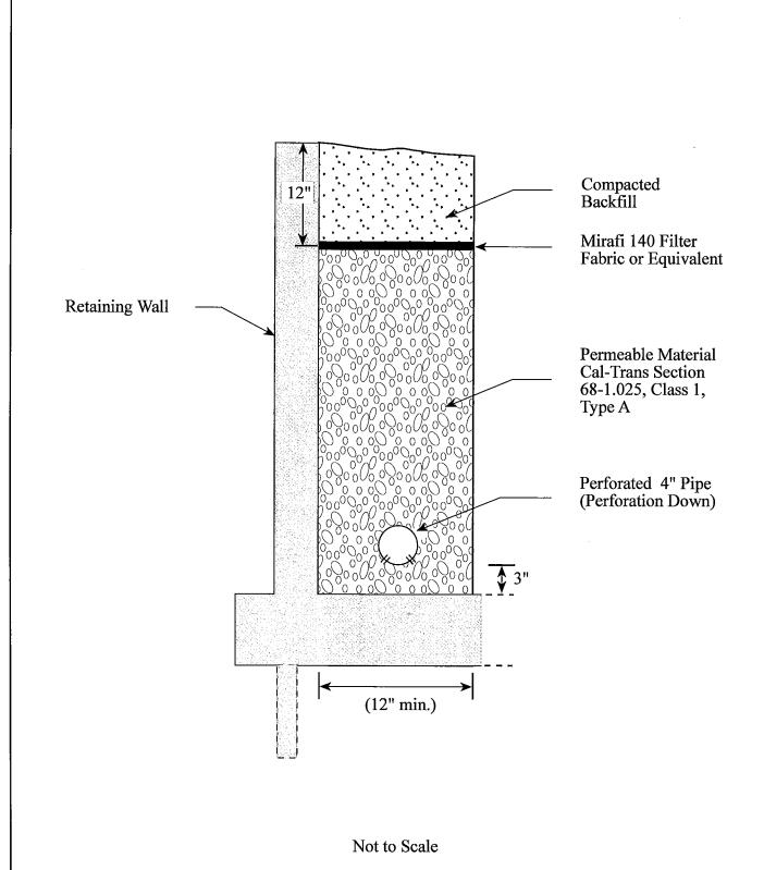
Pacific Crest Engineering Inc. 444 Airport Blvd., Suite 106 Watsonville, CA 95076 Typical Retaining Wall Drain Detail Electrical & Chemical Feed Building Seaside, California
