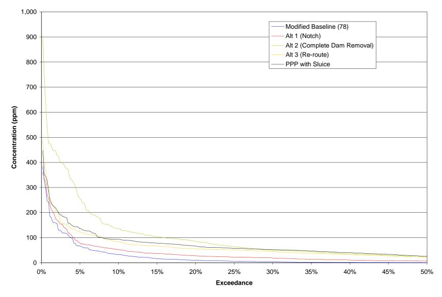
Figure P-2: Simulated Suspended Sediment Concentration Exceedance at Reach 4.7 for a Wet Year
