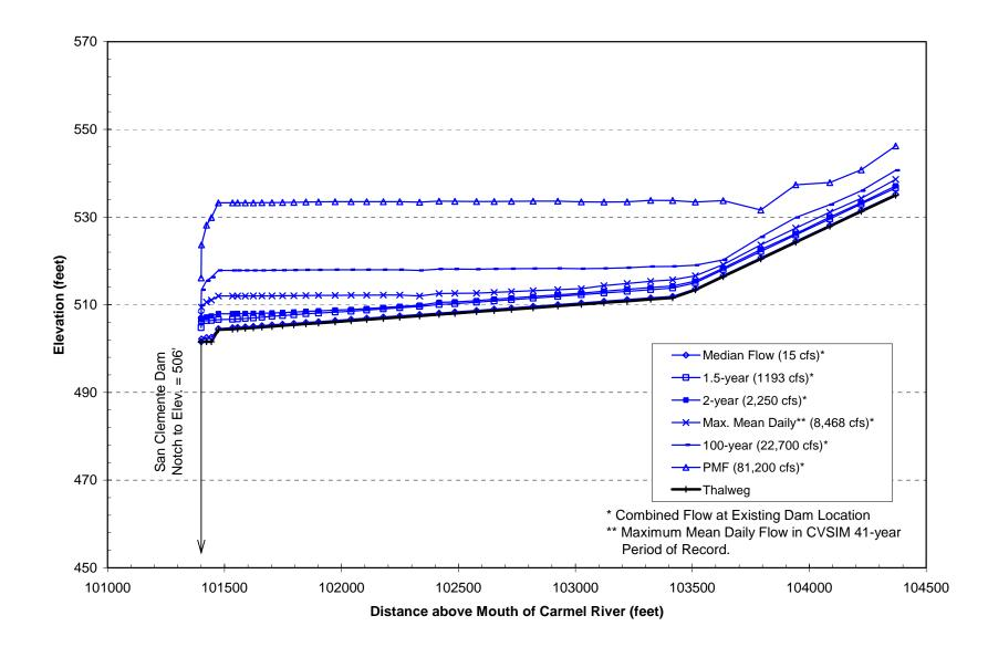
Figure 19. Computed water-surface profiles for selected discharges in the San Clemente Creek Branch of San Clemente Reservoir under the Notching Alternative.
