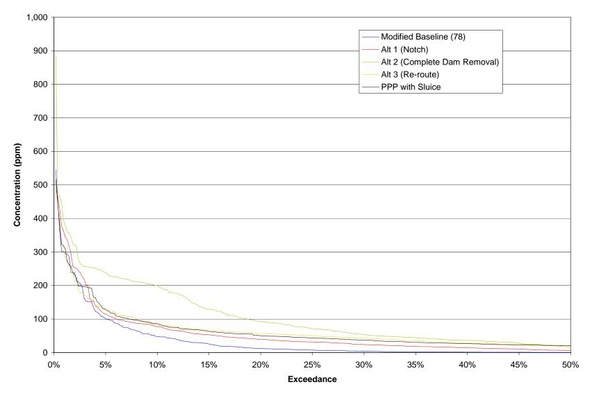
Figure P-4: Simulated Suspended Sediment Concentration Exceedance at Reach 6.3 for a Wet Year
