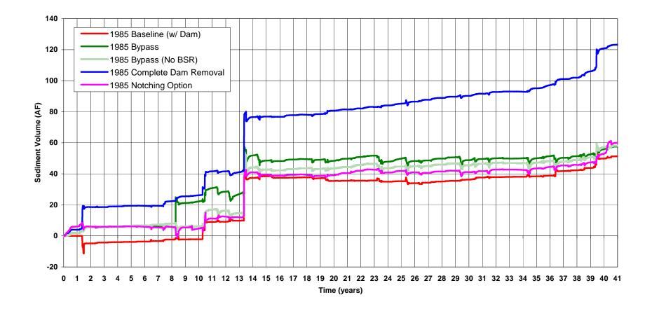
Figure 33. Total volume of sediment stored in the Carmel River downstream from San Clemente Dam for the 41-year simulation under baseline (with dam) conditions evaluated in MEI (2005) and for the Alternatives evaluated in this study (1985 start date).
