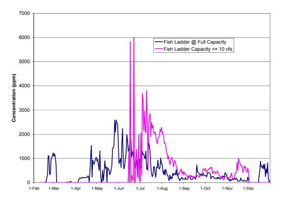
Figure 25. Total sediment concentrations in the fish ladder under the Proposed Project for the 1985 hydrology scenario with the fish ladder operating at full capacity, and with the fish ladder capacity restricted to 10 cfs or less.
