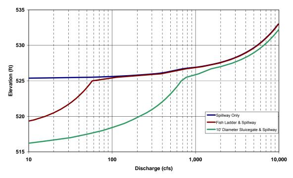
Figure 2. Hydraulic capacity rating curves for the principal spillway at San Clemente Dam, the combined fish ladder and spillway capacity, and the 10-foot diameter sluice gate and spillway.
