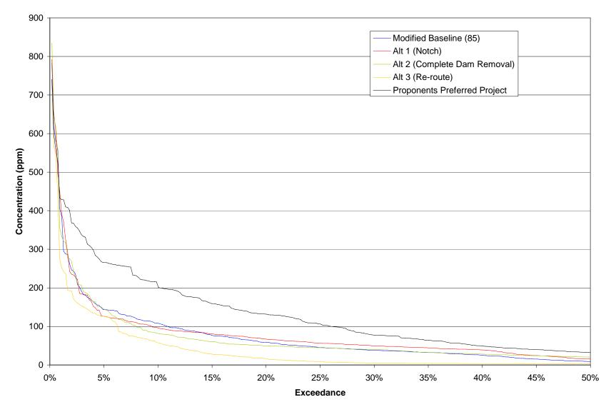
Figure P-12: Simulated Suspended Sediment Concentration Exceedance at Reach 4.7 for a Dry Year
