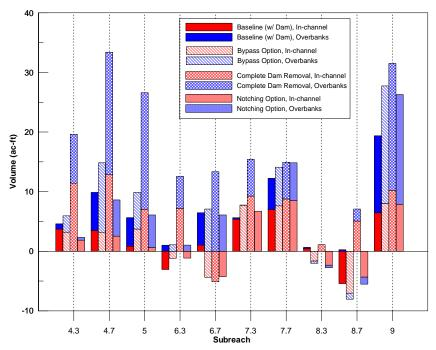
Figure 35a. Sediment volume stored in the river downstream from San Clemente Dam at the end of the 41-year simulation, by subreach, for the baseline (with dam) conditions evaluated in MEI (2005) and for the alternatives evaluated in this study (1978 start-date).
