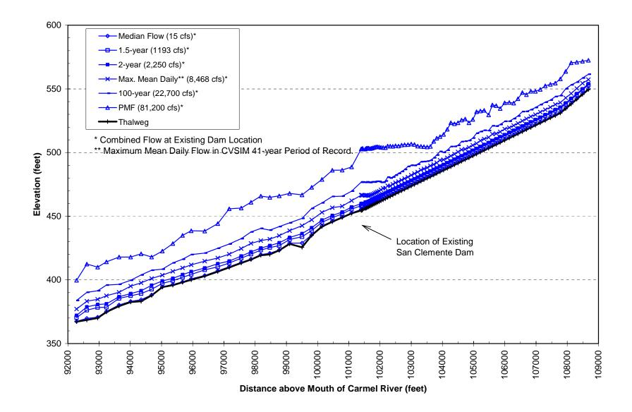
Figure 14. Computed water-surface profiles for selected discharges in the Carmel Branch of San Clemente Reservoir under the Complete Dam Removal Alternative.
