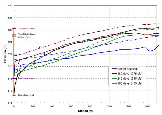
Figure 5d. Longitudinal profile of the incised channel upstream from the sluice gage at the end of the sluicing event, and 180, 240 and 360 days after the sluicing event, 1978 hydrology.
