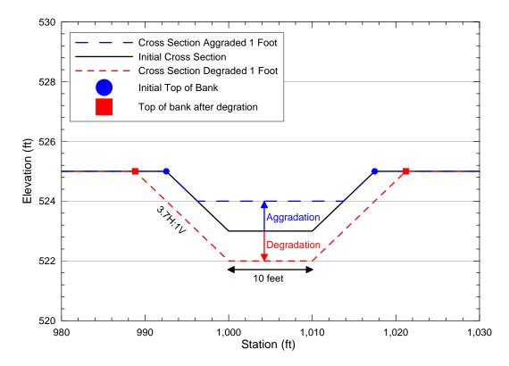
Figure 10. Conceptual sketch of channel modifications that were applied in the model during degradation and aggradation.
