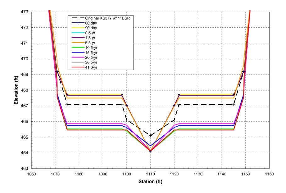
Figure 28. Typical cross section in the reconstructed reach of San Clemente Creek showing erosion of sediments in excess of 1.0 feet in the overbanks.
