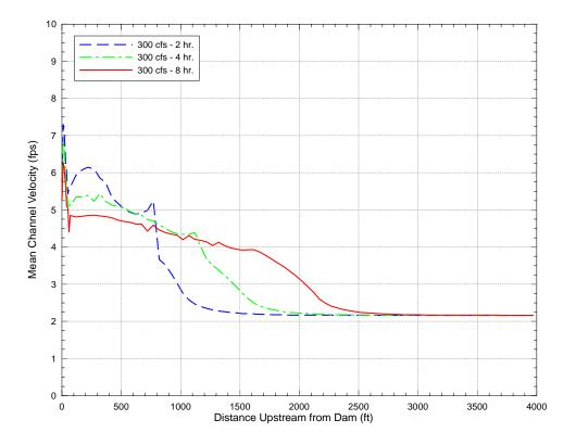
Figure 25. Cross-sectionally averaged velocity profiles at 2, 4, and 8 hours for a constant sluicing discharge of 300 cfs.
