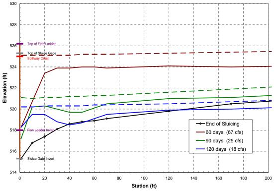
Figure 15c-1. Longitudinal profile of the incised channel upstream from the sluice gage at the end of the sluicing event, and 60, 90 and 120 days after the sluicing event, 1985 hydrology with fish ladder at full capacity, zoomed in on the downstream 200 feet of the incised channel.
