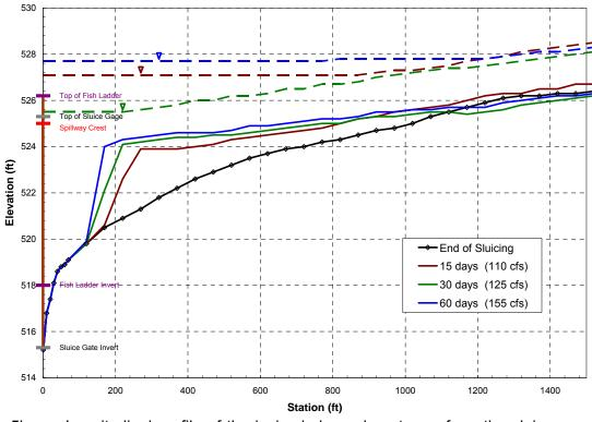
Figure 5b. Longitudinal profile of the incised channel upstream from the sluice gage at the end of the sluicing event, and 15, 30 and 60 days after the sluicing event, 1978 hydrology.
