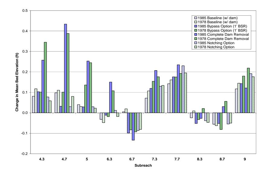
Figure 38. Change in mean bed elevation at the end of the simulation for each of the subreaches under the baseline (with dam) conditions evaluated in MEI (2005) and under the alternatives evaluated in this study.
