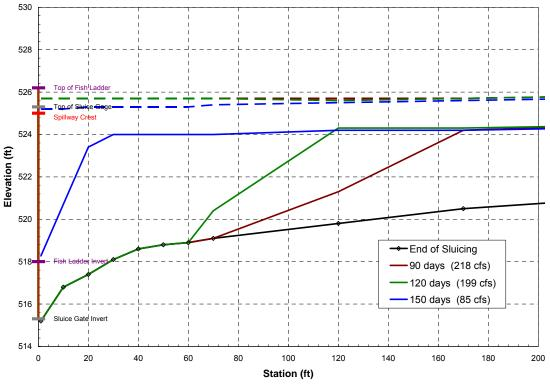
Figure 5c-1. Longitudinal profile of the incised channel upstream from the sluice gage at the end of the sluicing event, and 90, 120 and 150 days after the sluicing event, 1978 hydrology, zoomed in on the downstream 200 feet of the incised channel.
