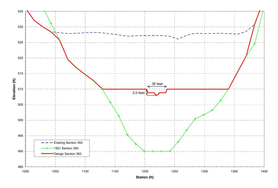
Figure 13. Typical cross section and design channel geometry for the reconstructed reach of the San Clemente Creek Branch under the Notching Alternative.
