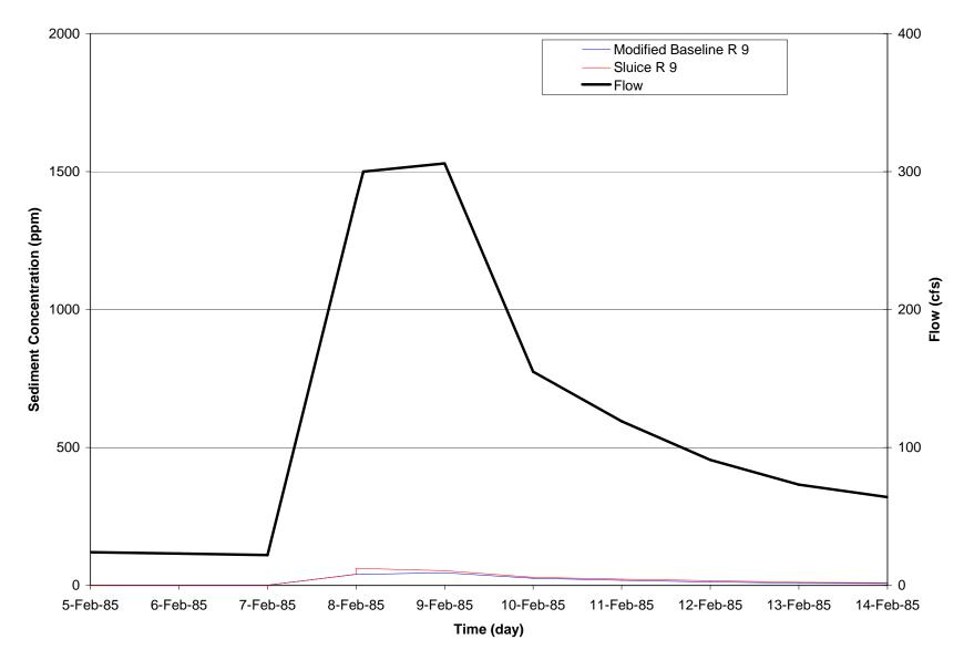
Figure O-24: Simulated Suspended Sediment Concentration at Reach 9 for a Dry Year
