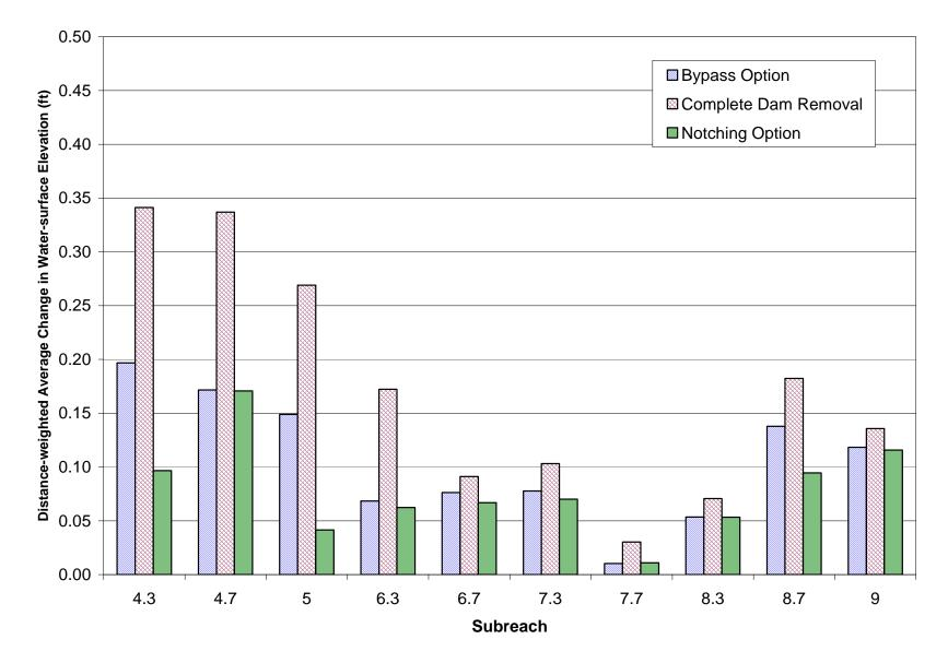
Figure 41. Distance-weighted average difference in maximum 100-year water-surface elevation from existing conditions, by subreach, for the alternatives evaluated in this study (1978 start date).
