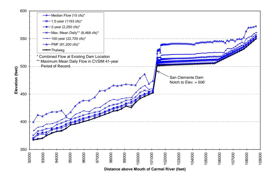
Figure 18. Computed water-surface profiles for selected discharges in the Carmel Branch of San Clemente Reservoir under the Notching Alternative.
