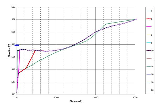
Figure 28. Profile of the incised channel 2 to 20 days after the end of sluicing operations at a constant discharge through the fish ladder of 40 cfs.
