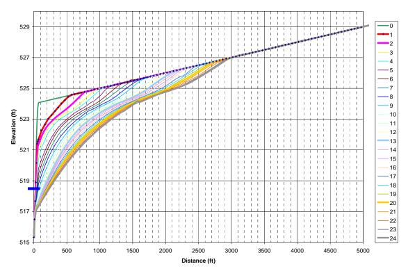
Figure 13. Estimated longitudinal profiles of the incised channel upstream from the sluice gate in 1-hour increments at a constant sluicing discharge of 100 cfs. Blue mark is water-surface elevation at sluice gate inlet.
