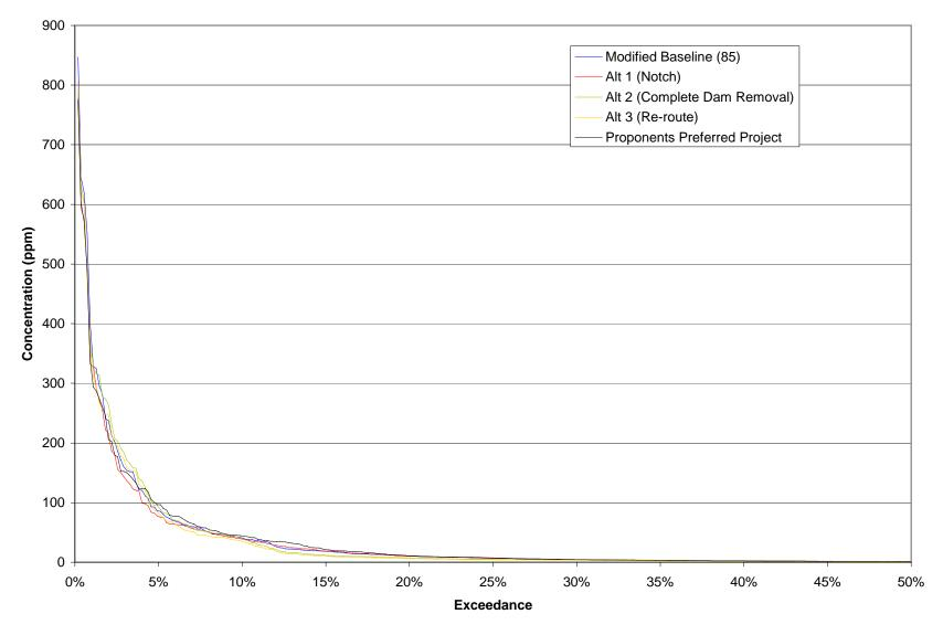
Figure P-18: Simulated Suspended Sediment Concentration Exceedance at Reach 8.3 for a Dry Year
