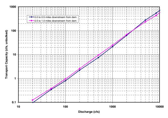
Figure 18. Sediment-transport capacity rating curves for the first two 0.5-mile segments of the Carmel River downstream from San Clemente Dam.
