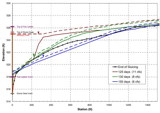
Figure 21c. Longitudinal profile of the incised channel upstream from the sluice gage at the end of the sluicing event, and 125, 130 and 150 days after the sluicing event, 1985 hydrology with fish ladder restricted to 10 cfs or less.
