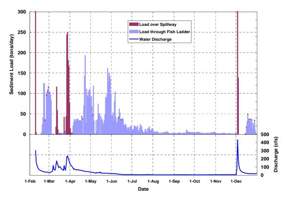
Figure 16. Sediment loads passing over the San Clemente Dam Spillway and through the fish ladder for the 1985 simulation. Also shown is the mean daily flow hydrograph for the simulation period.
