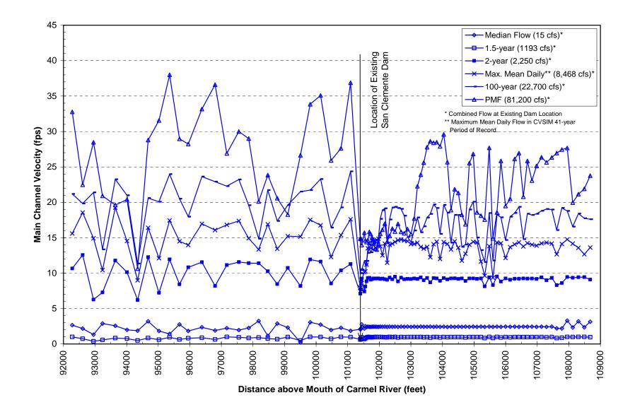
Figure 16. Computed main-channel velocity profiles for selected discharges in the Carmel River Branch of San Clemente Reservoir under the Complete Dam Removal Alternative.
