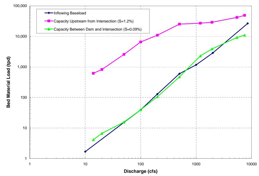
Figure 11. Inflowing sediment load (base load) and computed transport capacity of the reconstructed reach of the Carmel River between the dam and the intersection with the pre-dam surface.
