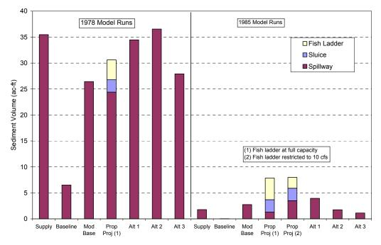
Figure 7. Total sediment volume passing San Clemente Dam between the date of the sluicing event (January 4, 1978; February 9, 1985) and the end of the calendar year for baseline, modified baseline (full reservoir), Proponents Proposed project, and Alternatives 1, 2 and 3 for 1985 and 1978 model runs. Also shown is the total upstream sediment supply to the reservoir.
