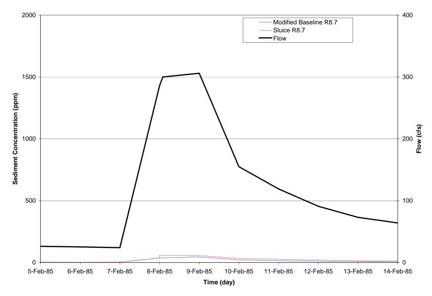
Figure O-23: Simulated Suspended Sediment Concentration at Reach 8.7 for a Dry Year
