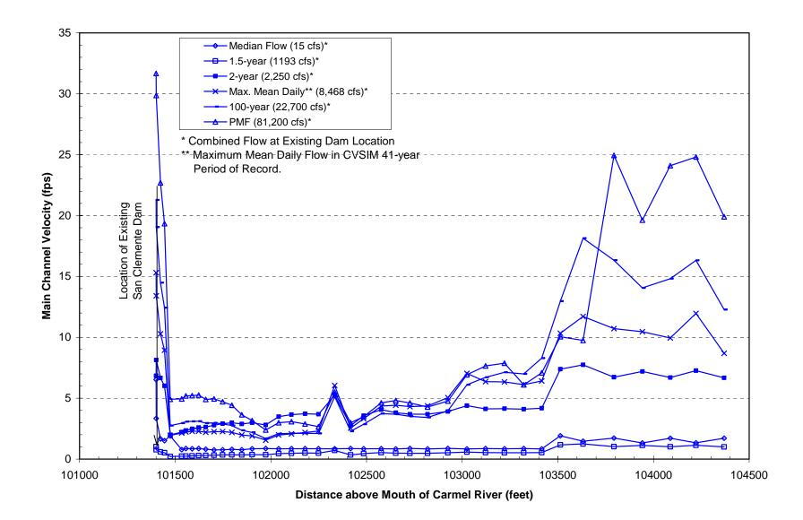
Figure 21. Computed main-channel velocity profiles for selected discharges in the San Clemente Creek Branch of San Clemente Reservoir under the Notching Alternative.
