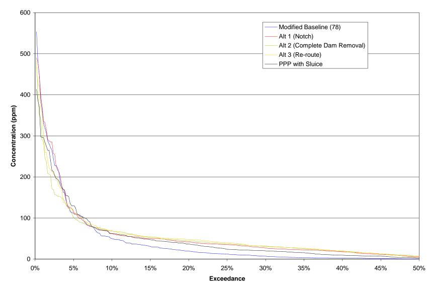
Figure P-7: Simulated Suspended Sediment Concentration Exceedance at Reach 7.7 for a Wet Year
