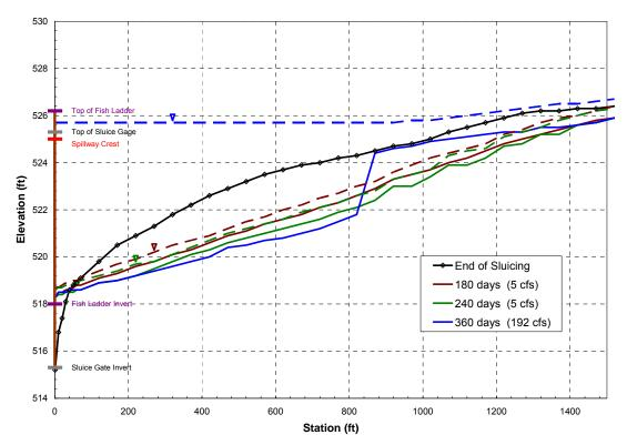
Figure 21d. Longitudinal profile of the incised channel upstream from the sluice gage at the end of the sluicing event, and 180, 240 and 360 days after the sluicing event, 1985 hydrology with fish ladder restricted to 10 cfs or less.
