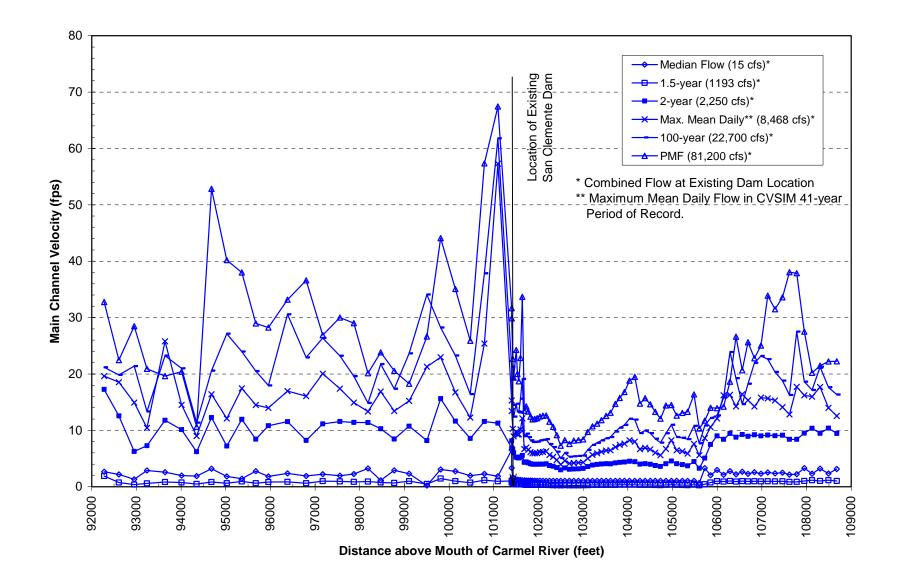
Figure 20. Computed main-channel velocity profiles for selected discharges in the Carmel Branch of San Clemente Reservoir under the Notching Alternative.
