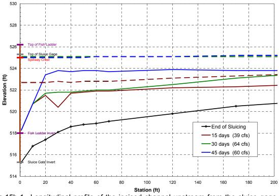
Figure 15b-1. Longitudinal profile of the incised channel upstream from the sluice gage at the end of the sluicing event, and 15, 30 and 45 days after the sluicing event, 1985 hydrology with fish ladder at full capacity, zoomed in on the downstream 200 feet of the incised channel.
