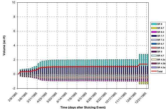
Figure 19. Change in sediment storage in the Carmel River downstream from San Clemente Dam, by subreach, from February 9 through December 31 for the 1985 hydrology for the modified baseline (full reservoir) scenario.
