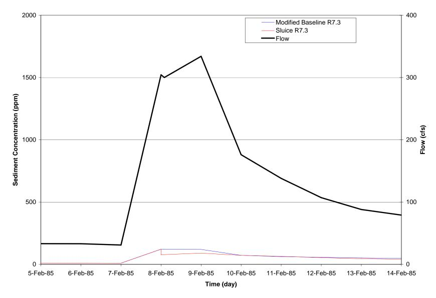
Figure O-20: Simulated Suspended Sediment Concentration at Reach 7.3 for a Dry Year
