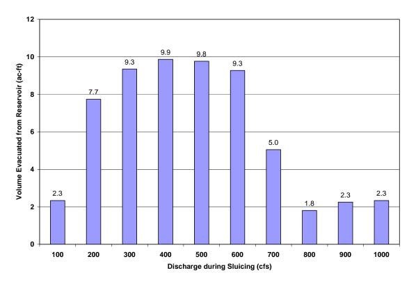
Figure 11. Total volume of sediment eroded from the reservoir deposits and passed into the downstream river after 24 hours at constant discharges ranging from 100 to 1,000 cfs.
