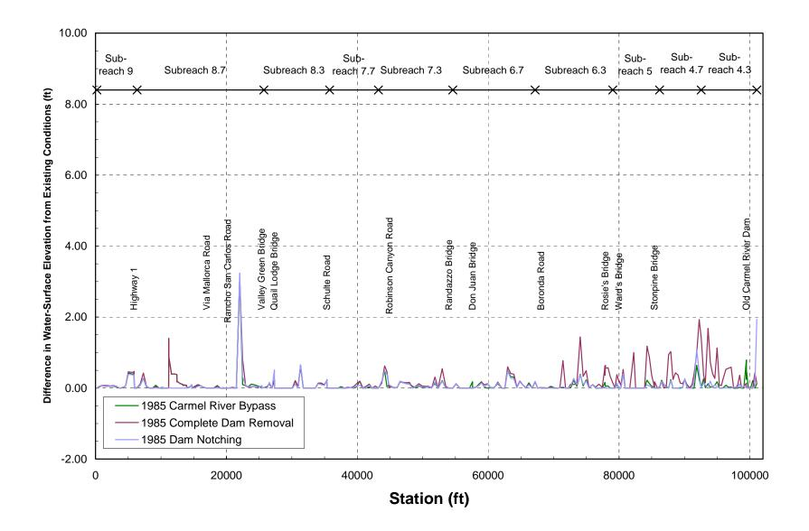
Figure 40. Maximum difference in 100-year water-surface elevation from existing conditions for the alternatives evaluated in this study (1985 start date).
