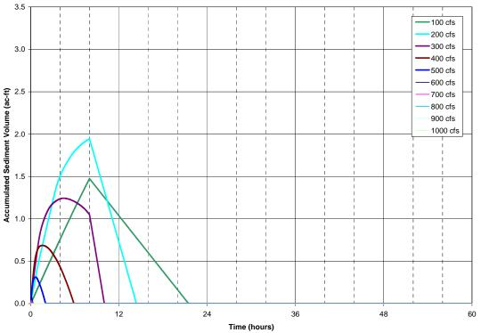
Figure 20. Volume of sediment accumulated in the 0.5-mile reach of the Carmel River immediately downstream from the dam for an 8-hour sluicing operation at discharges ranging from 100 to 1,000 cfs.
