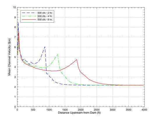
Figure 26. Cross-sectionally averaged velocity profiles at 2, 4, and 8 hours for a constant sluicing discharge of 500 cfs
