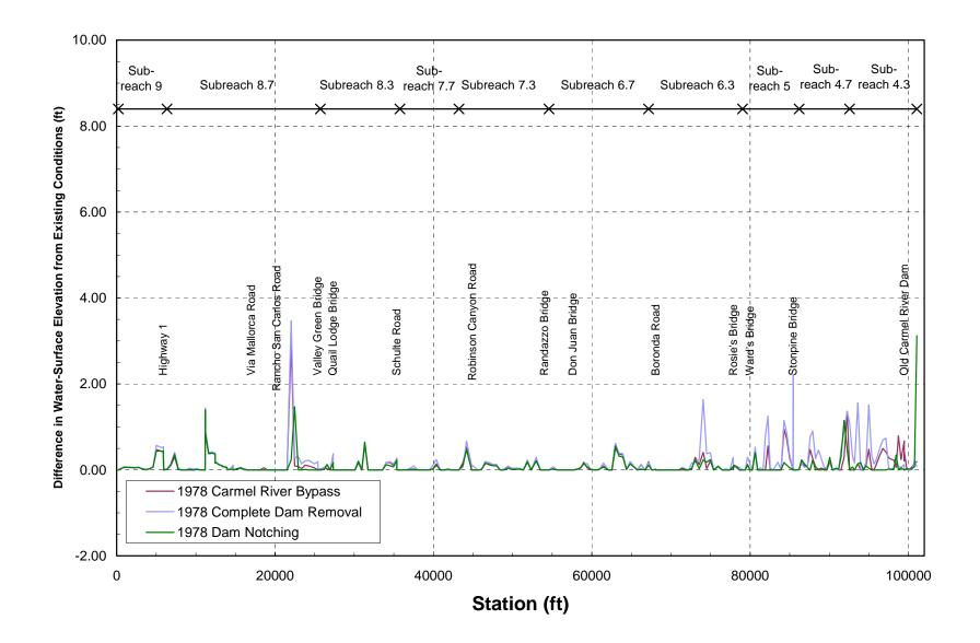
Figure 39. Maximum difference in 100-year water-surface elevation from existing conditions for the alternatives evaluated in this study (1978 start date).
