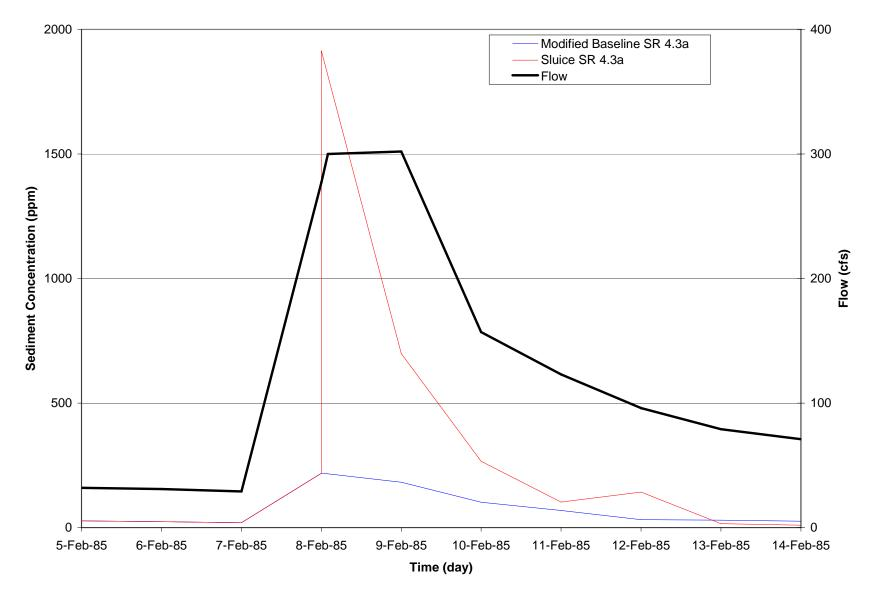
Figure O-15: Simulated Suspended Sediment Concentration at Reach 4.3 for a Dry Year
