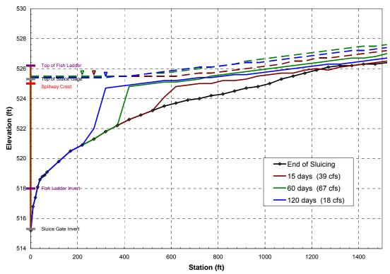
Figure 21b. Longitudinal profile of the incised channel upstream from the sluice gage at the end of the sluicing event, and 15, 60 and 120 days after the sluicing event, 1985 hydrology with fish ladder restricted to 10 cfs or less.
