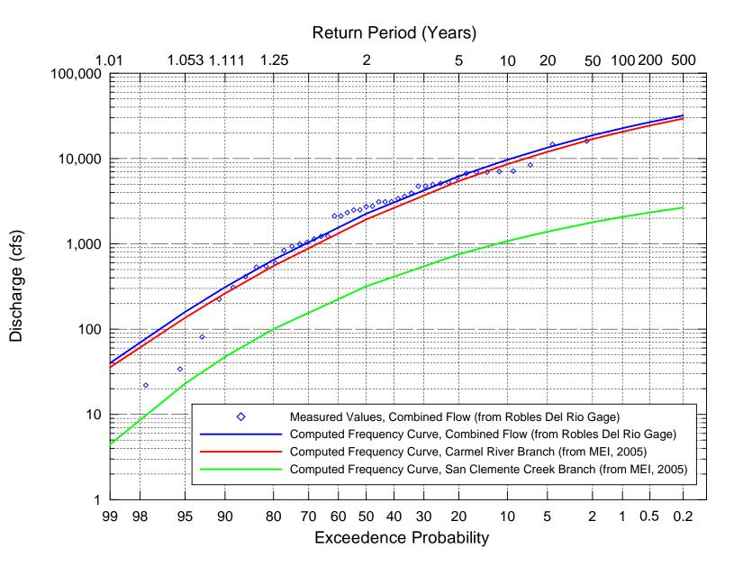
Figure 12. Computed peak flood-frequency curve for the combined flow (based on the Robles Del Rio flood-frequency analysis), and for the Carmel River and San Clemente Creek Branches of San Clemente Reservoir (as discussed in MEI, 2005).
