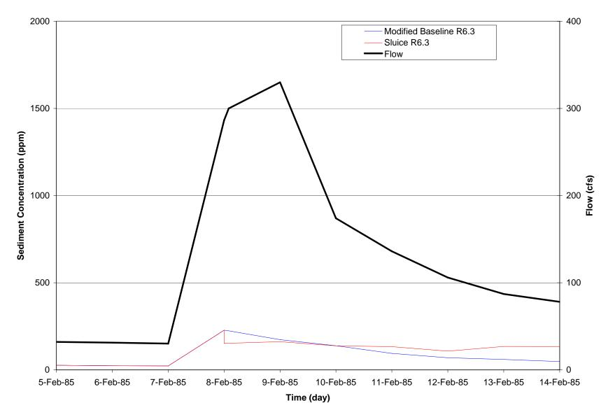
Figure O-18: Simulated Suspended Sediment Concentration at Reach 6.3 for a Dry Year
