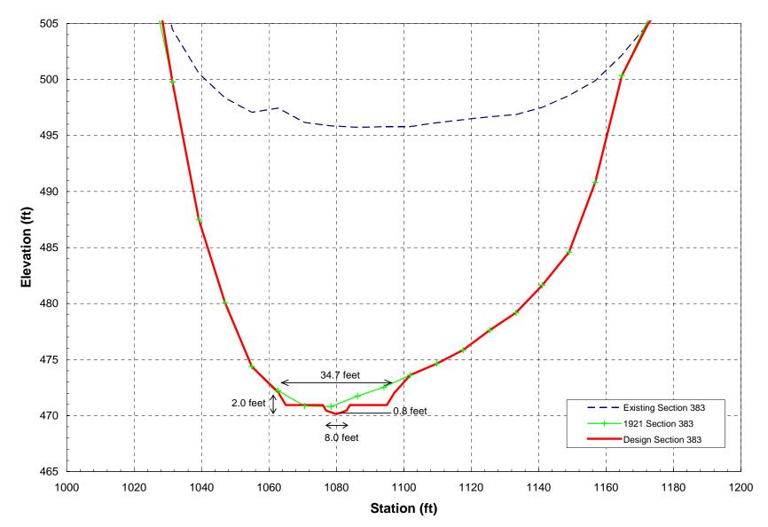
Figure 8. Typical cross section and design channel geometry for the reconstructed reach of the San Clemente Creek Branch under the Complete Dam Removal Alternative.
