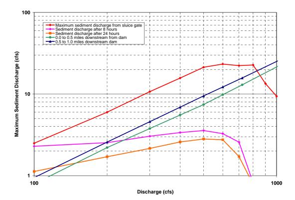
Figure 19. Sediment discharge passing through the sluice gate near the beginning of sluicing operations (maximum discharge curve), after 8 hours and after 24 hours of sluicing. Also shown are the transport capacity rating curves for the two 0.5-mile segments of river immediately downstream from the dam.
