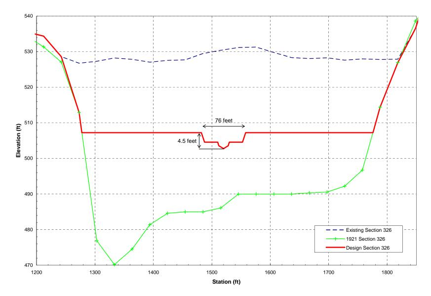
Figure 10. Typical cross section and design channel geometry (downstream from the intersection with the pre-dam surface) for the reconstructed reach of the Carmel Branch under the Notching Alternative.
