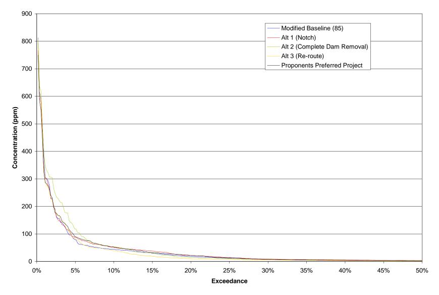
Figure P-17: Simulated Suspended Sediment Concentration Exceedance at Reach 7.7 for a Dry Year
