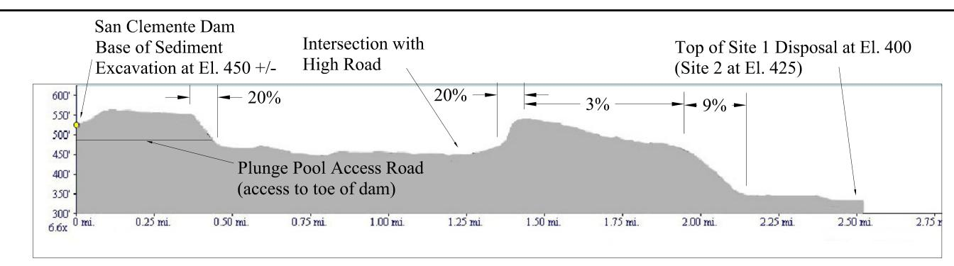
Site 1 Profile - Conveyor/Slurry Route (via Plunge Pool Access Road, San Clemente Drive, and Pipeline Access Road
