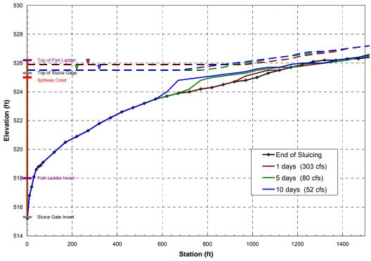
Figure 21a. Longitudinal profile of the incised channel upstream from the sluice gage at the end of the sluicing event, and 1, 5 and 10 days after the sluicing event, 1985 hydrology with fish ladder restricted to 10 cfs or less.
