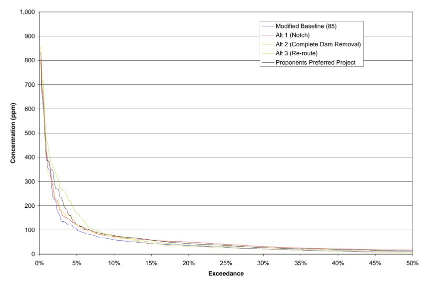
Figure P-16: Simulated Suspended Sediment Concentration Exceedance at Reach 7.3 for a Dry Year
