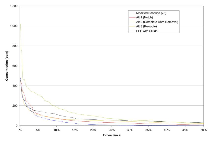
Figure P-3: Simulated Suspended Sediment Concentration Exceedance at Reach 5 for a Wet Year
