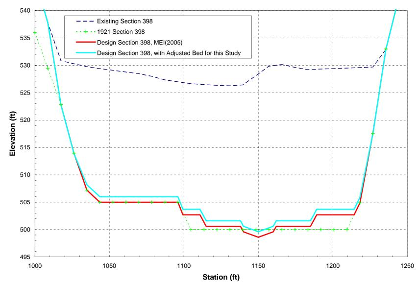
Figure 22. Typical cross section in the reconstructed reach of San Clemente Creek under the Carmel River Bypass Alternative showing the existing section, the pre-dam (1921) section, the design section (MEI, 2005), and the adjusted design section for this study.
