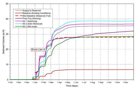
Figure 8. Cumulative sediment load passing San Clemente Dam from October 1, 1977, through December 31, 1978, for baseline and modified baseline (reservoir filled with sediment), Proponents Proposed Project, and Alternatives 1, 2 and 3).
