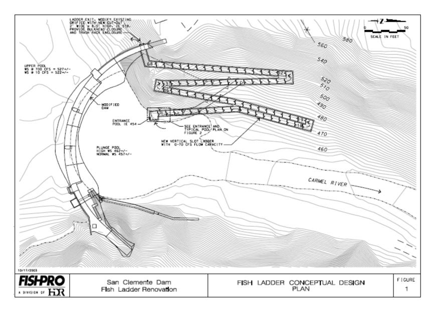
Figure 1. Fish ladder conceptual design, plan view of spillway and ladder exit (Figure 1 from FishPro and Entrix, 2003).
