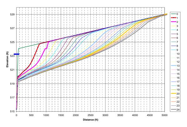
Figure 15. Estimated longitudinal profiles of the incised channel upstream from the sluice gate in 1-hour increments at a constant sluicing discharge of 500 cfs. Blue mark is water-surface elevation at sluice gate inlet.
