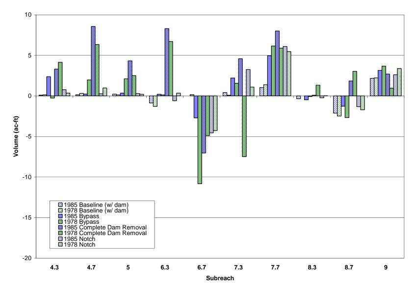
Figure 36. Volume of gravels stored in the main channel in each of the subreaches under the baseline (with dam) conditions evaluated in MEI (2005) and under the alternatives evaluated in this study.
