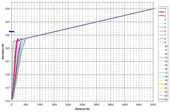
Figure 16. Estimated longitudinal profiles of the incised channel upstream from the sluice gate in 1-hour increments at a constant sluicing discharge of 800 cfs. Blue mark is water-surface elevation at sluice gate inlet.
