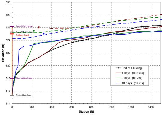
Figure 15a. Longitudinal profile of the incised channel upstream from the sluice gage at the end of the sluicing event, and 1, 5 and 10 days after the sluicing event, 1985 hydrology with fish ladder at full capacity.
