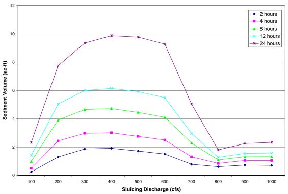
Figure 12. Volume of sediment delivered to the downstream river at constant discharge ranging from 100 to 1,000 cfs over sluicing durations of 2, 4, 8, 12, and 24 hours.
