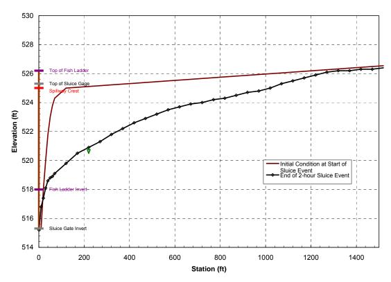
Figure 1. Assumed longitudinal profile of the sediment deposits in San Clemente Reservoir at the start of the sluicing event, and the simulated profiles after 2, 4, 8, and 24 hours of sluicing at a steady-state discharge of 300 cfs.
