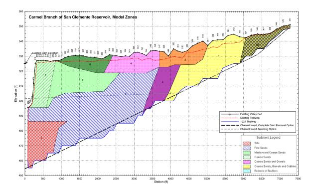
Figure 27. Profile of reservoir sediment zones and the channel invert for the Complete Dam Removal Alternative and for the Notching Alternative, Carmel Branch of San Clemente Reservoir.
