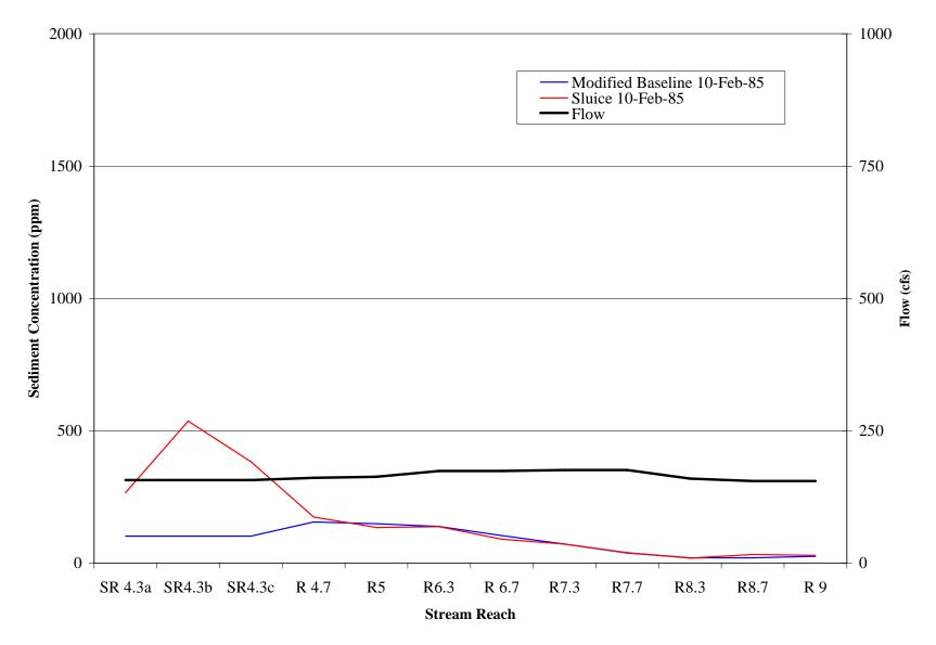
Figure O-27: Simulated Suspended Sediment Concentration along Carmel River for Day 3 of a Dry Year Sluice Event
