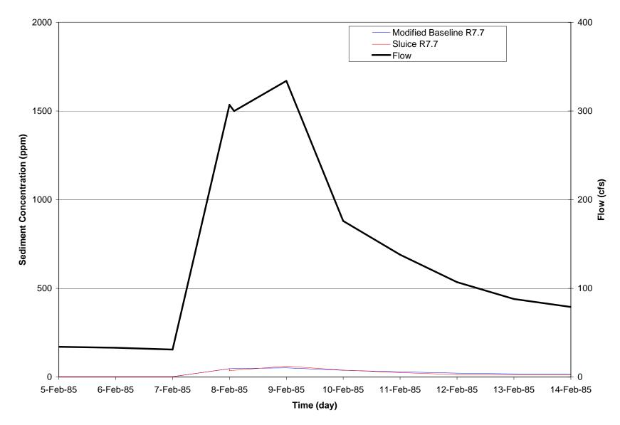
Figure O-21: Simulated Suspended Sediment Concentration at Reach 7.7 for a Dry Year
