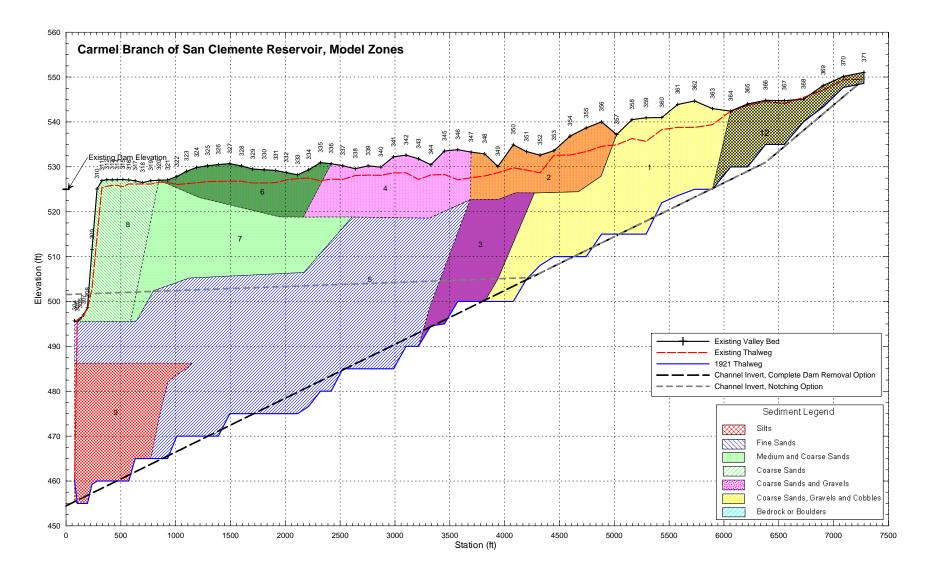
Figure 25. Profile of reservoir sediment zones and the channel invert for the Complete Dam Removal Alternative and for the Notching Alternative, Carmel Branch of San Clemente Reservoir.
