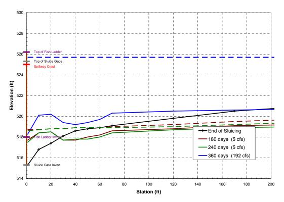
Figure 15d-1. Longitudinal profile of the incised channel upstream from the sluice gage at the end of the sluicing event, and 180, 240 and 360 days after the sluicing event, 1985 hydrology with fish ladder at full capacity, zoomed in on the downstream 200 feet of the incised channel.
