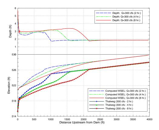
Figure 22. Simulated minimum bed elevation, water-surface elevation and maximum depth profiles at 2, 4, and 8 hours for a constant sluicing discharge of 300 cfs.
