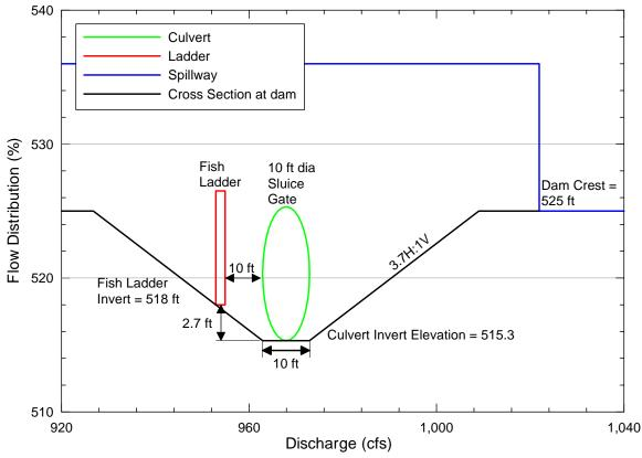
Figure 4. Conceptual sketch, looking downstream, of San Clemente Dam, the vertical slot fish ladder proposed by FishPro and Entrix (2003) and a 10-foot diameter sluice gate. Also shown is the approximate cross section of the channel upstream from the sluice gate when it has incised to the level of the sluice gate invert.
