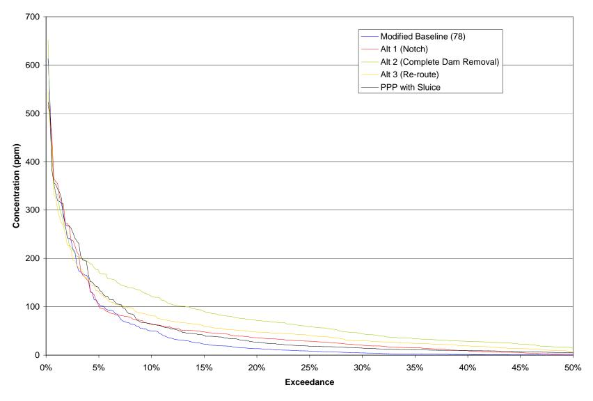
Figure P-5: Simulated Suspended Sediment Concentration Exceedance at Reach 6.7 for a Wet Year
