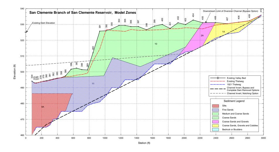
Figure 23. Profile of reservoir sediment zones and the channel invert for the Bypass, the Complete Dam Removal, and for the Notching Alternatives, San Clemente Creek Branch of San Clemente Reservoir.
