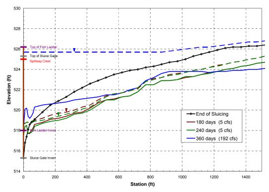
Figure 15d. Longitudinal profile of the incised channel upstream from the sluice gage at the end of the sluicing event, and 180, 240 and 360 days after the sluicing event, 1985 hydrology with fish ladder at full capacity.
