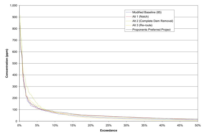
Figure P-15: Simulated Suspended Sediment Concentration Exceedance at Reach 6.7 for a Dry Year
