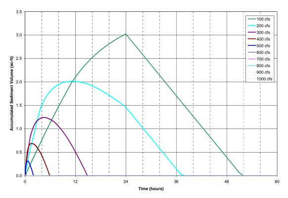
Figure 21. Volume of sediment accumulated in the 0.5-mile reach of the Carmel River immediately downstream from the dam for a 24-hour sluicing operation at discharges ranging from 100 to 1,000 cfs.
