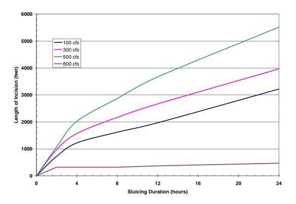
Figure 17. Estimated length of the incision upstream from the sluice gate at various points in the simulation at constant sluicing discharges of 100, 300, 500 and 800 cfs.
