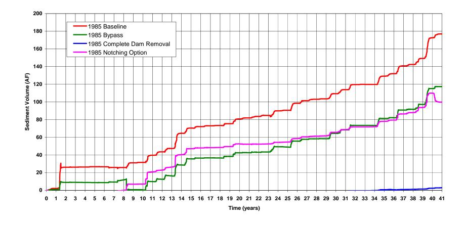
Figure 31. Total volume of sediment trapped in the reservoir (upstream of the existing dam) during the 41-year simulation for the baseline (with dam) conditions evaluated in MEI (2005) and for the Bypass, Complete Dam Removal, and Notching Alternatives in this study (1985 start date).
