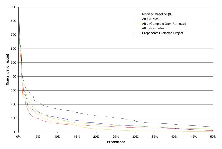
Figure P-13: Simulated Suspended Sediment Concentration Exceedance at Reach 5 for a Dry Year
