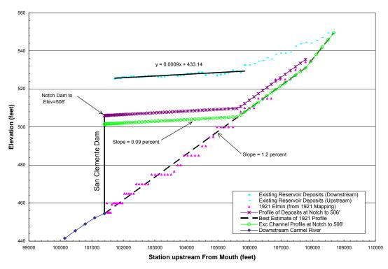
Figure 26. Longitudinal profile of the existing reservoir deposits, the pre-dam surface, and the constructed profile under the Notching Alternative in the Carmel Branch of San Clemente Reservoir.
