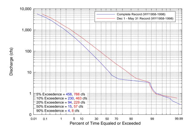
Figure 5. Mean daily flow-duration curve for the combined flows in the Carmel River and San Clemente Creek at San Clemente Dam for the full year and for the December 1 through May 31 fish-passage period, based on the CVSIM model results that were used to develop the 41-year period of record that was used in the previous sediment modeling studies (MEI, 2002 and 2003).
