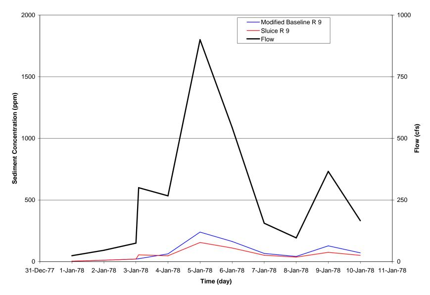
Figure O-10: Simulated Suspended Sediment Concentration at Reach 9 for a Wet Year
