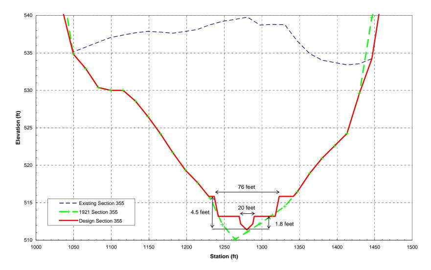
Figure 9. Typical cross section and design channel geometry (upstream from the intersection with the pre-dam surface) for the reconstructed reach of the Carmel Branch under the Notching Alternative.
