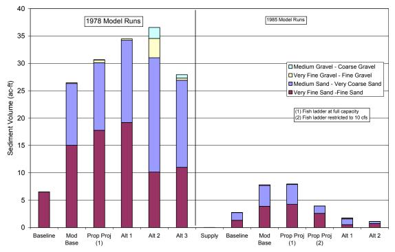
Figure 9. Size breakdown of sediment passing San Clemente Dam between the date of the sluicing event (January 4, 1978; February 9, 1985) and the end of the calendar year for baseline, modified baseline (full reservoir), Proponents Proposed project, and Alternatives 1, 2 and 3 for 1985 and 1978 model runs.
