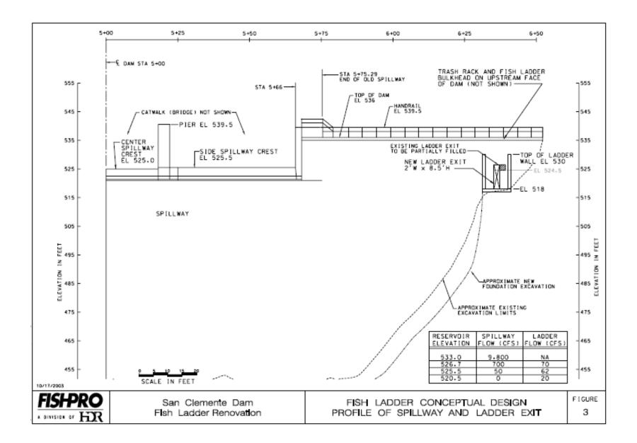
Figure 2. Fish ladder conceptual design, profile of spillway and ladder exit (Figure 3 from FishPro and Entrix, 2003).
