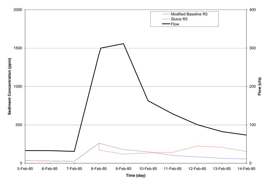
Figure O-17: Simulated Suspended Sediment Concentration at Reach 5 for a Dry Year
