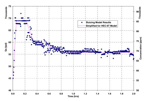
Figure 3. Sediment loads passing through the sluice gate during the 2-hour sluicing event from the sluicing model. Red line represents the sediment load-discharge relationship used in the HEC-6T model during the sluicing period.
