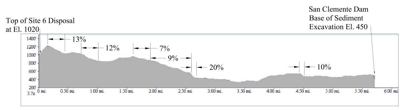
Profile of Conveyor/Slurry Route to Site 6R
