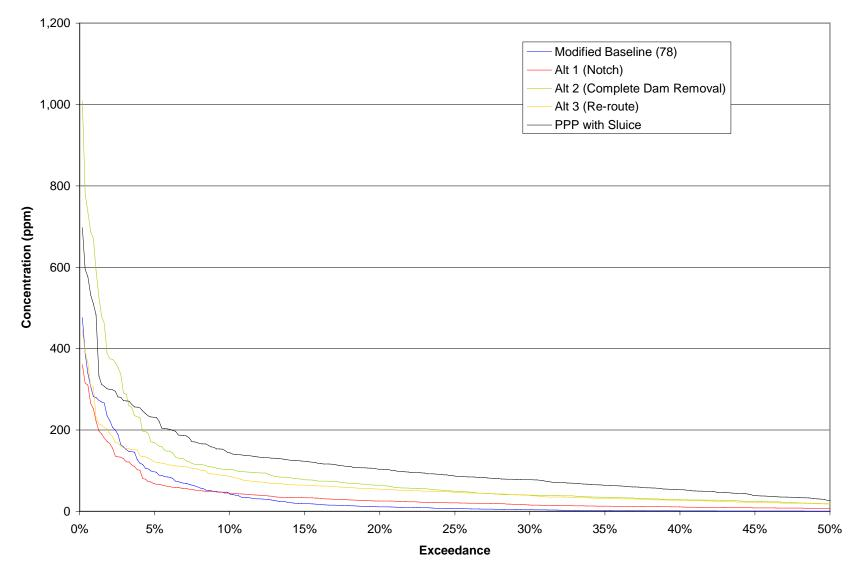
Figure P-1: Simulated Suspended Sediment Concentration Exceedance at Reach 4.3 for a Wet Year
