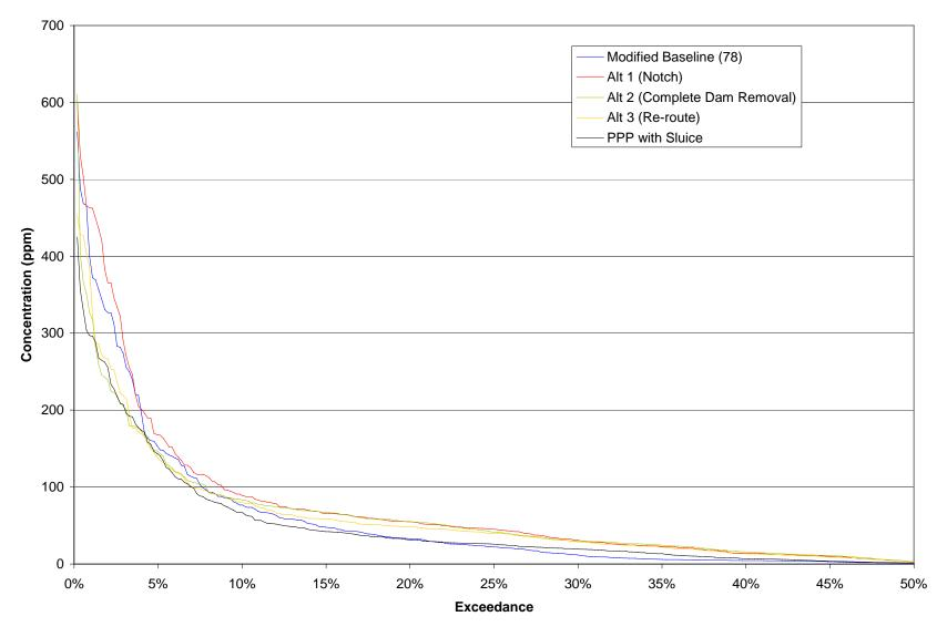
Figure P-10: Simulated Suspended Sediment Concentration Exceedance at Reach 9 for a Wet Year
