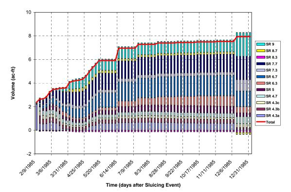
Figure 20. Change in sediment storage in the Carmel River downstream from San Clemente Dam, by subreach, from the end of the sluicing event on February 9 through December 31 for the 1985 hydrology for the Proponents Proposed Project (Sluicing), with the fish ladder operating at full capacity.
