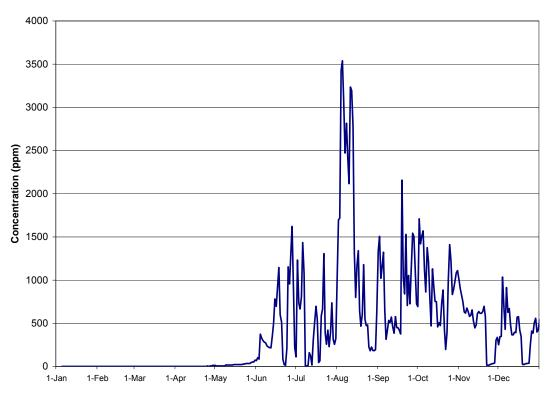
Figure 24. Total sediment concentrations in the fish ladder under the Proposed Project for the 1978 hydrology scenario.
