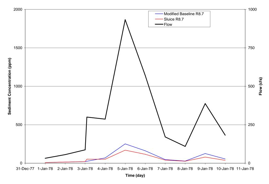
Figure O-9: Simulated Suspended Sediment Concentration at Reach 8.7 for a Wet Year
