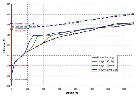
Figure 5a. Longitudinal profile of the incised channel upstream from the sluice gage at the end of the sluicing event, and 1, 5 and 10 days after the sluicing event, 1978 hydrology.
