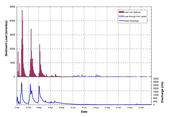
Figure 6. Sediment loads passing over the San Clemente Dam Spillway and through the fish ladder for the 1978 simulation. Also shown is the mean daily flow hydrograph for the simulation period.
