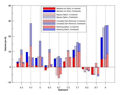
Figure 35b. Sediment volume stored in the river downstream from San Clemente Dam at the end of the 41-year simulation, by subreach, for the baseline (with dam) conditions evaluated in MEI (2005) and for the alternatives evaluated in this study (1985 start-date).
