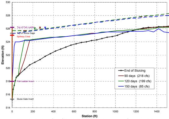
Figure 5c. Longitudinal profile of the incised channel upstream from the sluice gage at the end of the sluicing event, and 90, 120 and 150 days after the sluicing event, 1978 hydrology.
