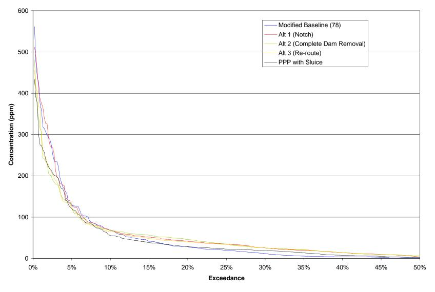
Figure P-9: Simulated Suspended Sediment Concentration Exceedance at Reach 8.7 for a Wet Year
