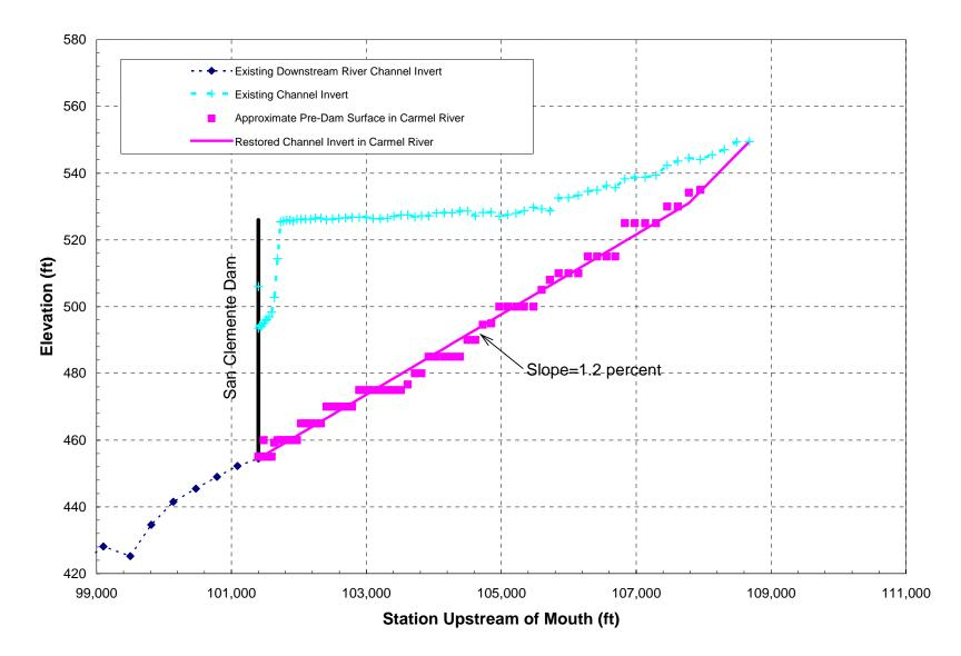
Figure 5. Profiles of the existing sediment deposits and reconstructed reach of the Carmel River Branch for the Complete Dam Removal Alternative.
