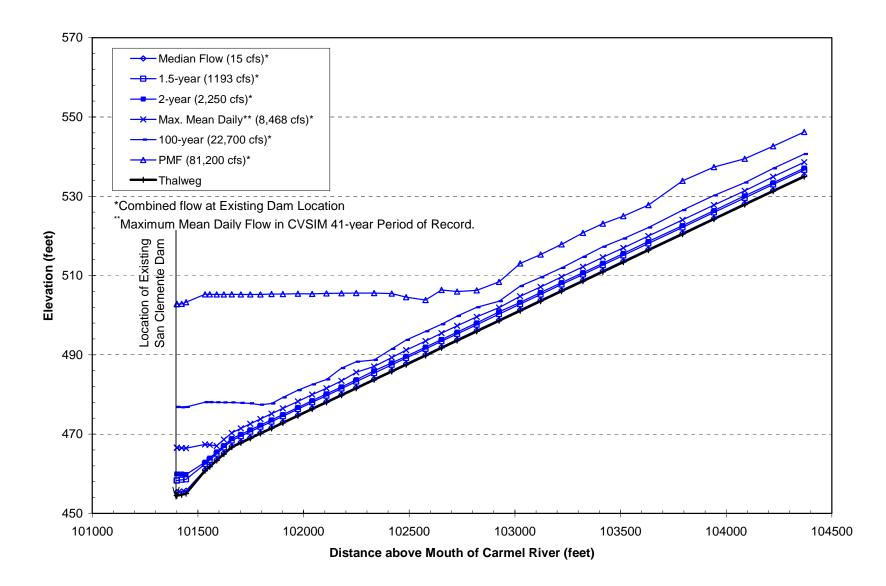
Figure 15. Computed water-surface profiles for selected discharges in the San Clemente Creek Branch of San Clemente Reservoir under the Complete Dam Removal Alternative.
