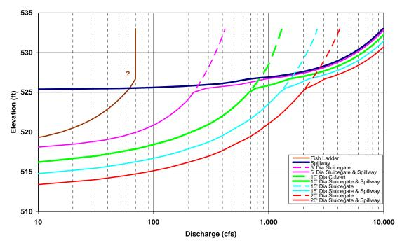
Figure 3. Hydraulic capacity rating curves for four potential sluice gate diameters (5, 10, 15, and 20 feet) and the principal spillway for the Dam Thickening Alternative. The hydraulic capacity rating curve for the fish ladder FishPro and Entrix (2003) is also shown.
