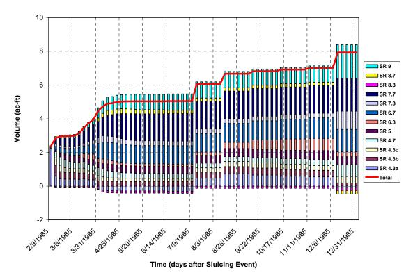
Figure 23. Change in sediment storage in the Carmel River downstream from San Clemente Dam, by subreach, from the end of the sluicing event on February 9 through December 31 for the 1985 hydrology for the Proponents Proposed Project (Sluicing), with the fish ladder restricted to 10 cfs or less.
