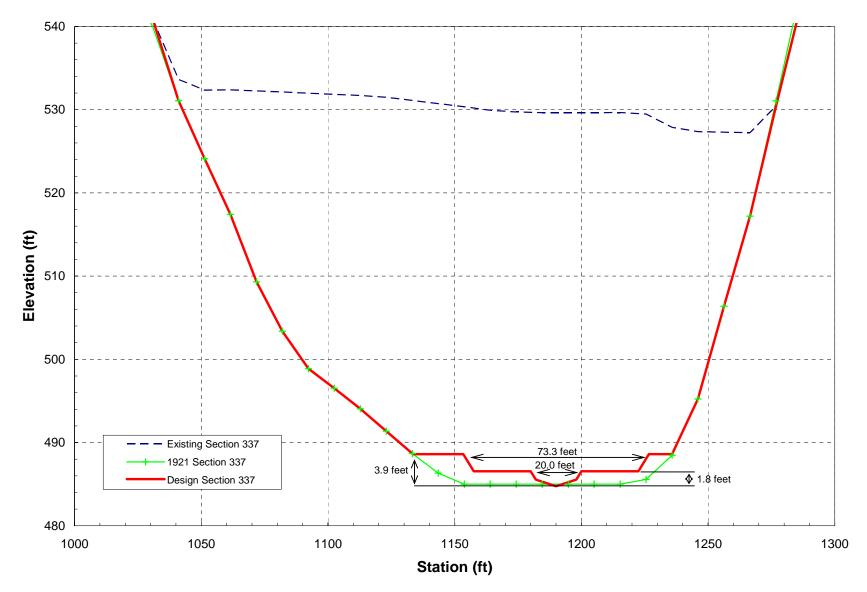
Figure 7. Typical cross section and design channel geometry for the reconstructed reach of the Carmel River Branch under the Complete Dam Removal Alternative.
