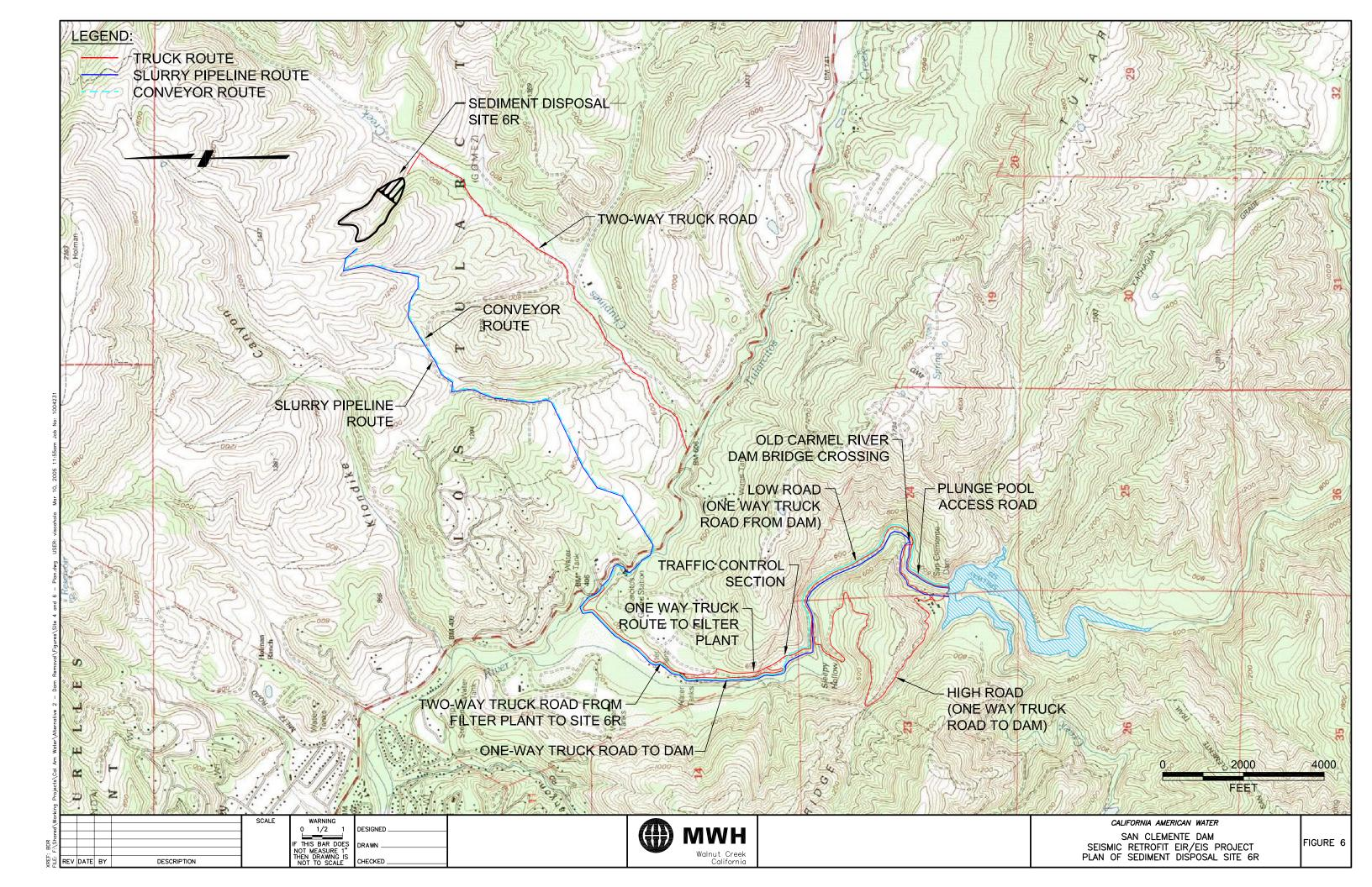
Three methods of sediment conveyance were identified for engineering screening: slurry pipeline, conveyor belt, and trucking.
