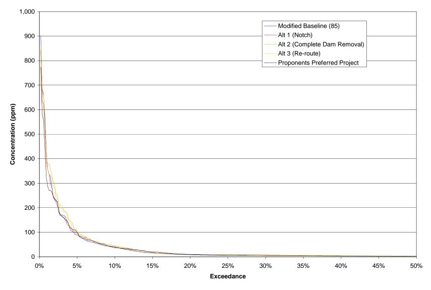
Figure P-19: Simulated Suspended Sediment Concentration Exceedance at Reach 8.7 for a Dry Year
