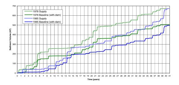
Figure 30. Inflowing Baseload and computed sediment load passing San Clemente Dam for baseline conditions (WY1978 and WY1985 start-dates).
