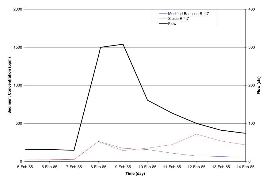
Figure O-16: Simulated Suspended Sediment Concentration at Reach 4.7 for a Dry Year
