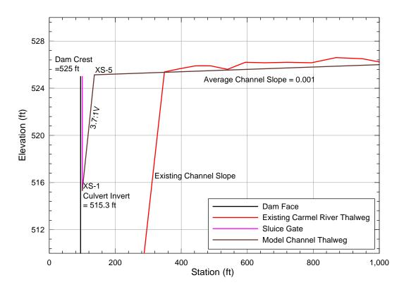
Figure 8. Longitudinal profile of the incised channel and reservoir sediment deposits that was assumed for the initial model conditions. Also shown for reference purposes is the profile of the existing reservoir deposits.
