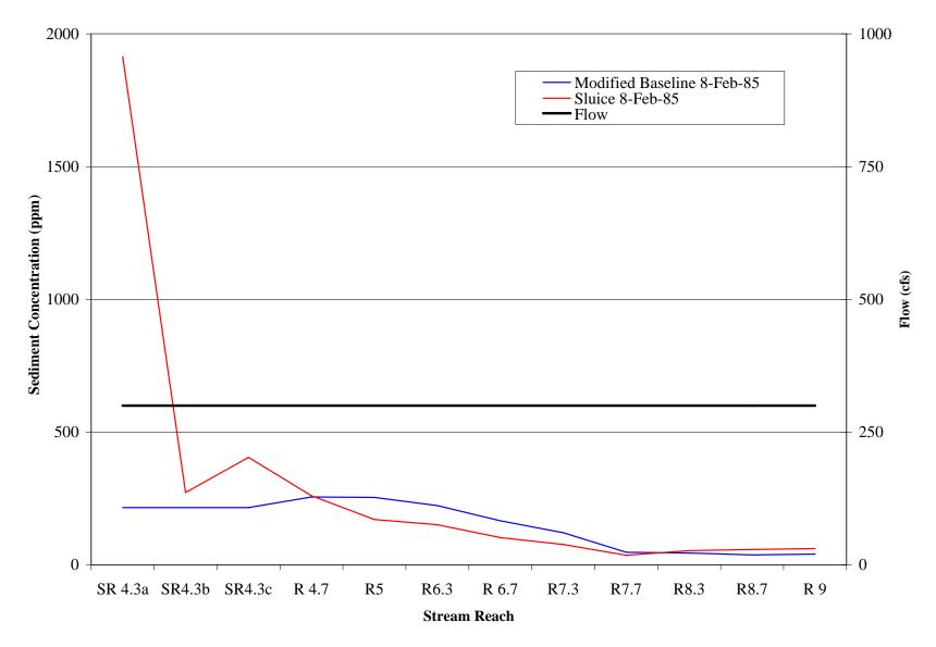
Figure O-25: Simulated Suspended Sediment Concentration along Carmel River for Day 1 of a Dry Year Sluice Event
