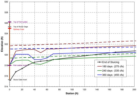
Figure 5d-1. Longitudinal profile of the incised channel upstream from the sluice gage at the end of the sluicing event, and 180, 240 and 360 days after the sluicing event, 1978 hydrology, zoomed in on the downstream 200 feet of the incised channel.
