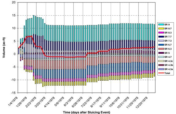
Figure 13. Change in sediment storage in the Carmel River downstream from San Clemente Dam, by subreach, from the end of the sluicing event on January 4 through December 31 for the 1978 hydrology for the Proponents Proposed Project (Sluicing).
