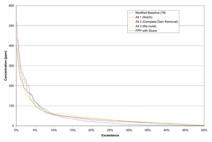
Figure P-8: Simulated Suspended Sediment Concentration Exceedance at Reach 8.3 for a Wet Year
