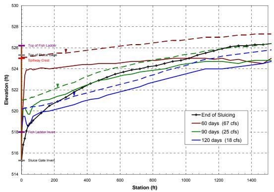
Figure 15c. Longitudinal profile of the incised channel upstream from the sluice gage at the end of the sluicing event, and 60, 90 and 120 days after the sluicing event, 1985 hydrology with fish ladder at full capacity.
