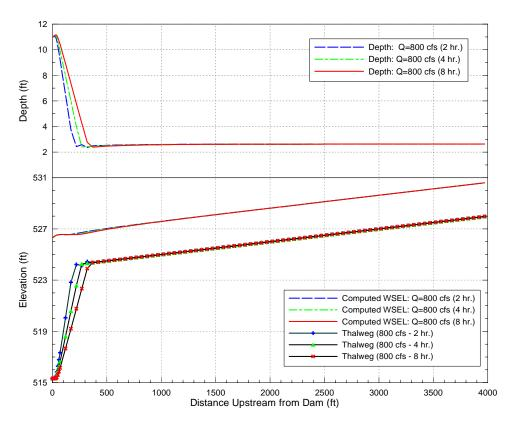
Figure 24. Simulated minimum bed elevation, water-surface elevation and maximum depth profiles at 2, 4, and 8 hours for a constant sluicing discharge of 800 cfs.
