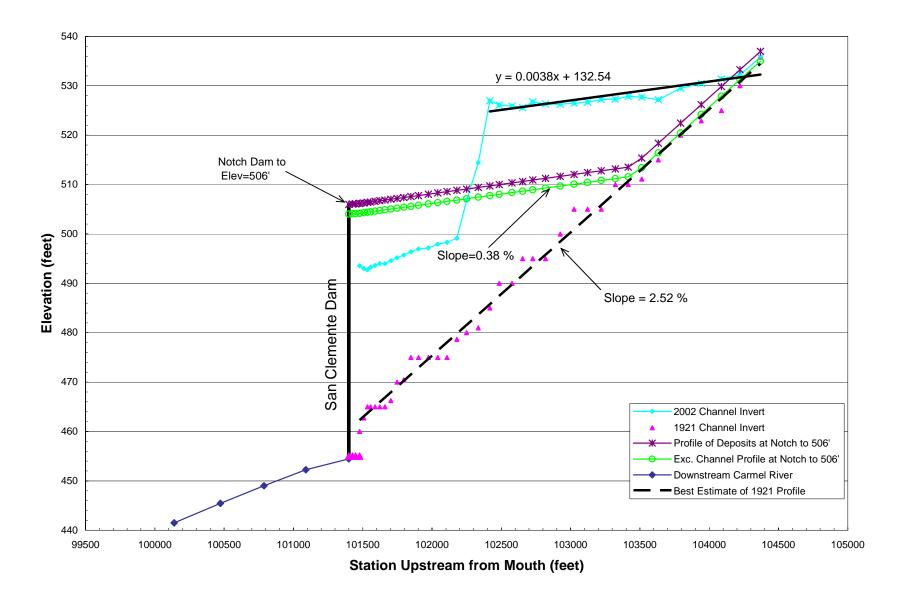
Figure 4. Longitudinal profile of the existing reservoir deposits, the pre-dam surface, and the constructed profile under the Notching Alternative in the San Clemente Creek Branch of San Clemente Reservoir.
