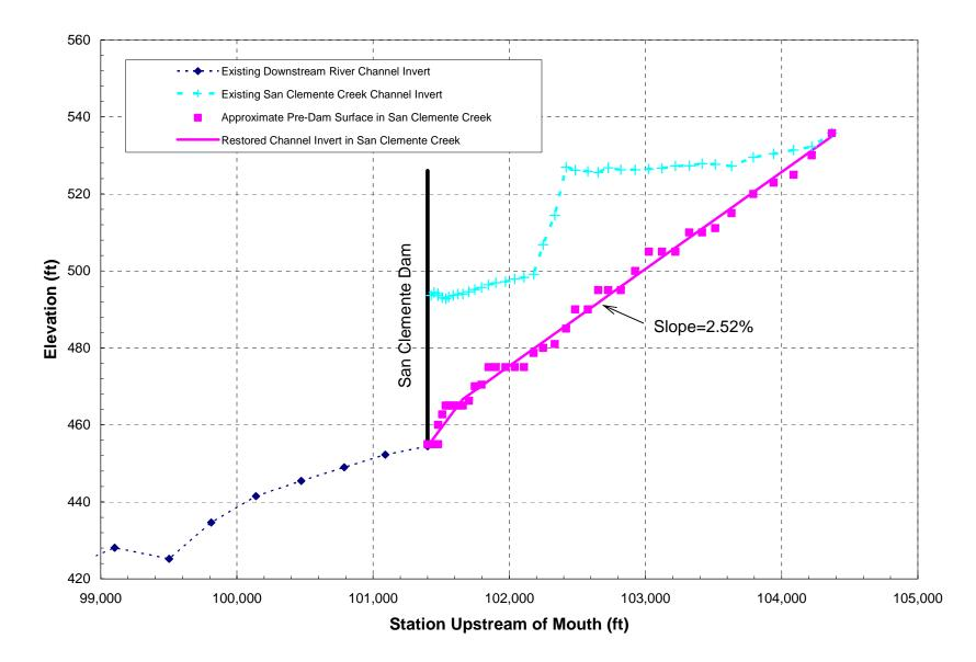
Figure 6. Profiles of the existing sediment deposits and reconstructed reach of the San Clemente Creek Branch for the Complete Dam Removal Alternative.
