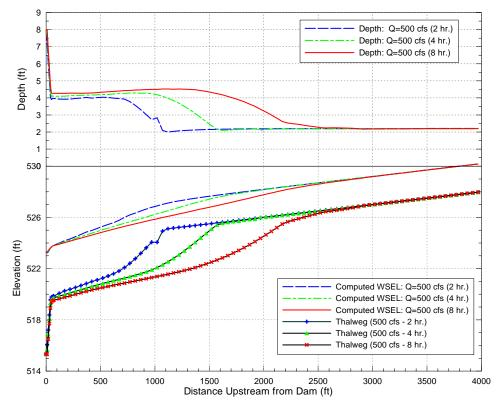
Figure 23. Simulated minimum bed elevation, water-surface elevation and maximum depth profiles at 2, 4, and 8 hours for a constant sluicing discharge of 500 cfs.
