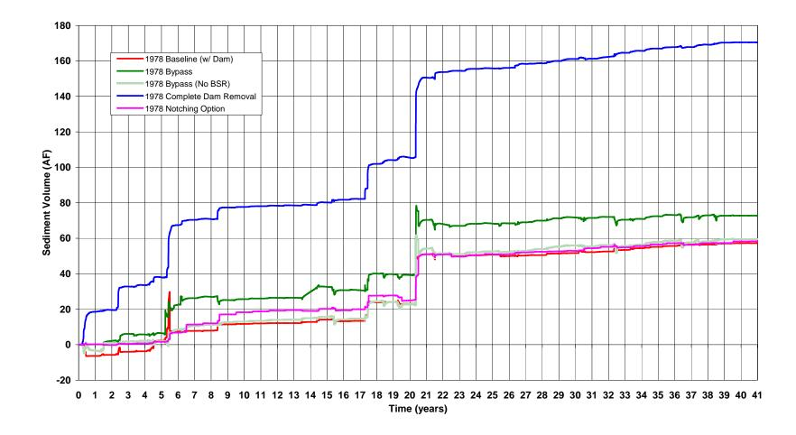
Figure 32. Total volume of sediment stored in the Carmel River downstream from San Clemente Dam for the 41-year simulation under baseline (with dam) conditions evaluated in MEI (2005) and for the Alternatives evaluated in this study (1978 start date).
