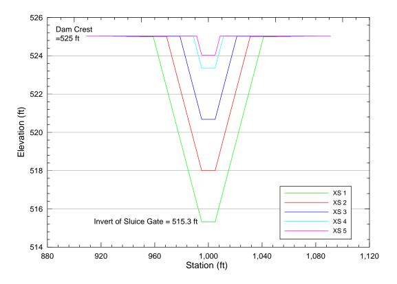
Figure 9. Geometry of initial cross sections immediately upstream from the sluice gate.
