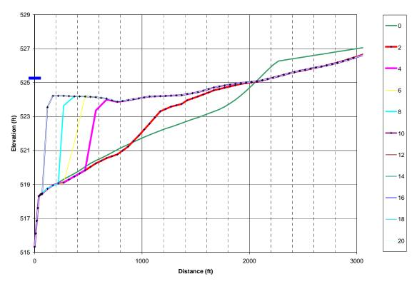
Figure 29. Profile of the incised channel 2 to 20 days after the end of sluicing operations at a constant discharge through the fish ladder of 60 cfs.
