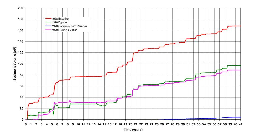
Figure 30. Total volume of sediment trapped in the reservoir (upstream of the existing dam) during the 41-year simulation for the baseline (with dam) conditions evaluated in MEI (2005) and for the Bypass, Complete Dam Removal, and Notching Alternatives in this study (1978 start date).
