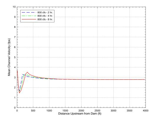
Figure 27. Cross-sectionally averaged velocity profiles at 2, 4, and 8 hours for a constant sluicing discharge of 800 cfs.
