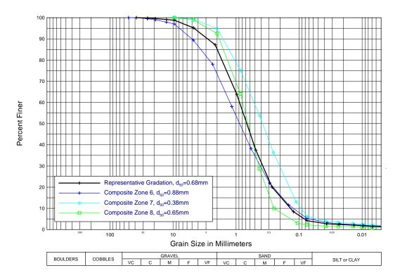
Figure 7. Representative sediment gradation for the sluicing analysis developed from the weighted average of Composite Zones 6, 7 and 8 shown in Figure 6.
