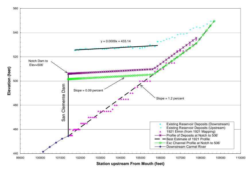
Figure 3. Longitudinal profile of the existing reservoir deposits, the pre-dam surface, and the constructed profile under the Notching Alternative in the Carmel Branch of San Clemente Reservoir.
