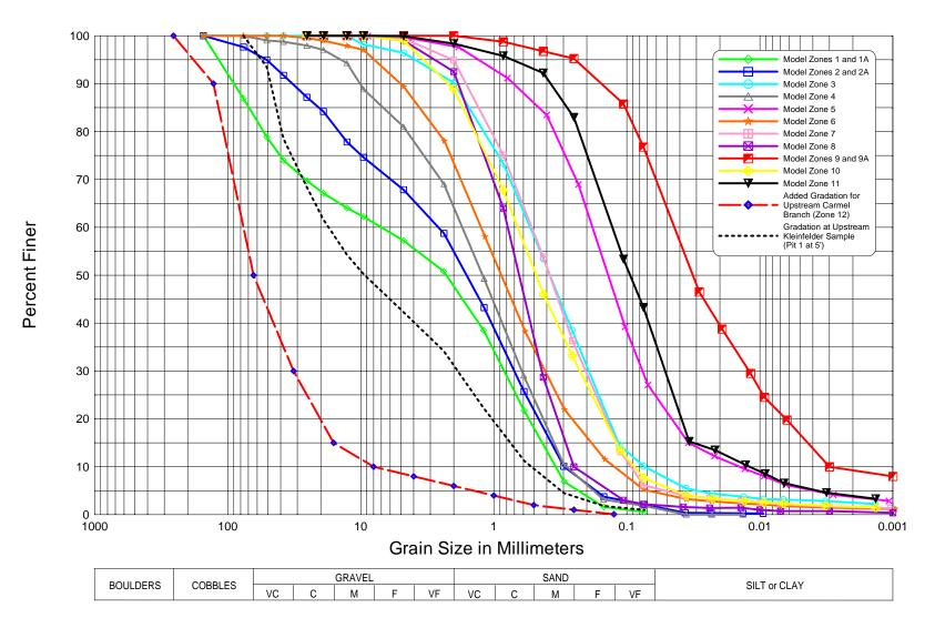
Figure 24. Gradation curves for the model sediment zones (from MEI, 2005).
