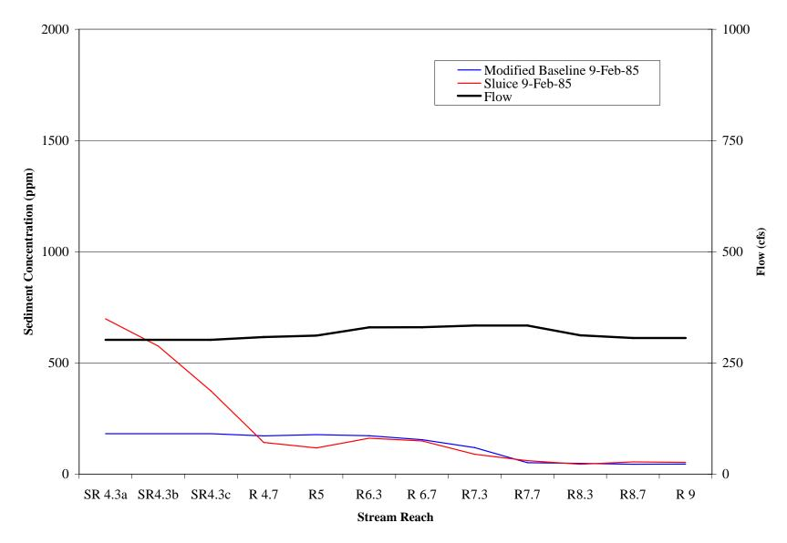
Figure O-26: Simulated Suspended Sediment Concentration along Carmel River for Day 2 of a Dry Year Sluice Event
