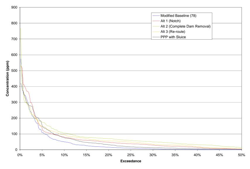
Figure P-6: Simulated Suspended Sediment Concentration Exceedance at Reach 7.3 for a Wet Year
