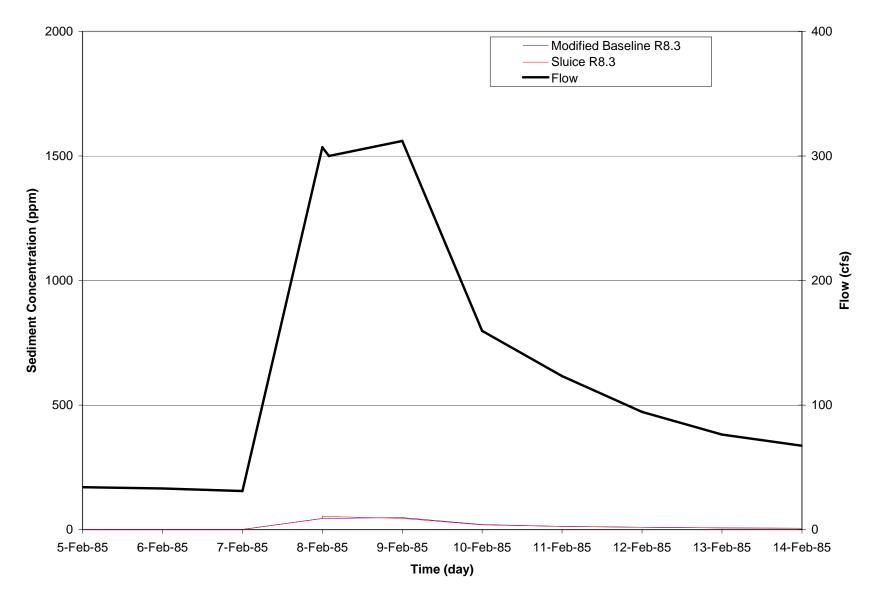
Figure O-22: Simulated Suspended Sediment Concentration at Reach 8.3 for a Dry Year
