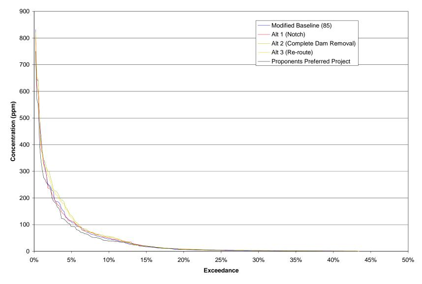
Figure B-20: Simulated Suspended Sediment Concentration Exceedance at Reach 9 for a Dry Year
