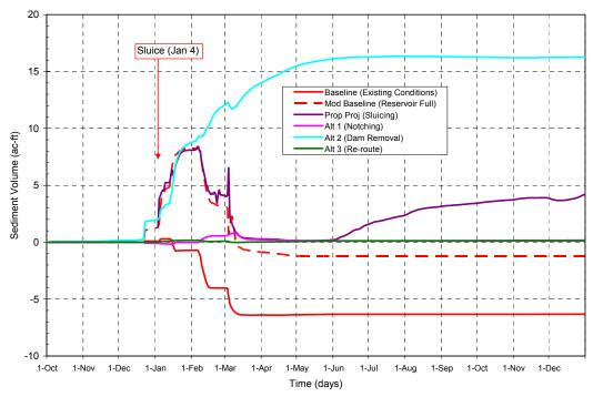
Figure 10. Change in sediment storage in the Carmel River between San Clemente Dam and the mouth between October 1, 1977, through December 31, 1978, for baseline and modified baseline (reservoir filled with sediment), Proponents Proposed Project, and Alternatives 1, 2 and 3).
