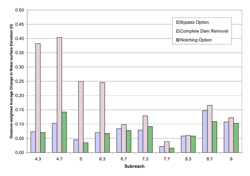
Figure 42. Distance-weighted average difference in maximum 100-year water-surface elevation from existing conditions, by subreach, for the alternatives evaluated in this study (1985 start date).
