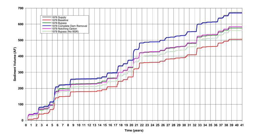
Figure 26. Inflowing base load and estimated sediment load passing the location of the existing dam for baseline (with dam) conditions evaluated in MEI (2005) and for the Bypass, Complete Dam Removal, and Notching Alternatives evaluated in this study (1978 start date). Also shown are the results from the Bypass Alternative with no BSR evaluated in MEI (2005) for the 1978 start date.
