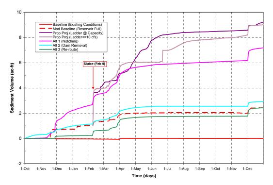
Figure 18. Change in sediment storage in the Carmel River between San Clemente Dam and the mouth between October 1, 1985, through December 31, 1985, for baseline and modified baseline (reservoir filled with sediment), Proponents Proposed Project, and Alternatives 1, 2 and 3).
