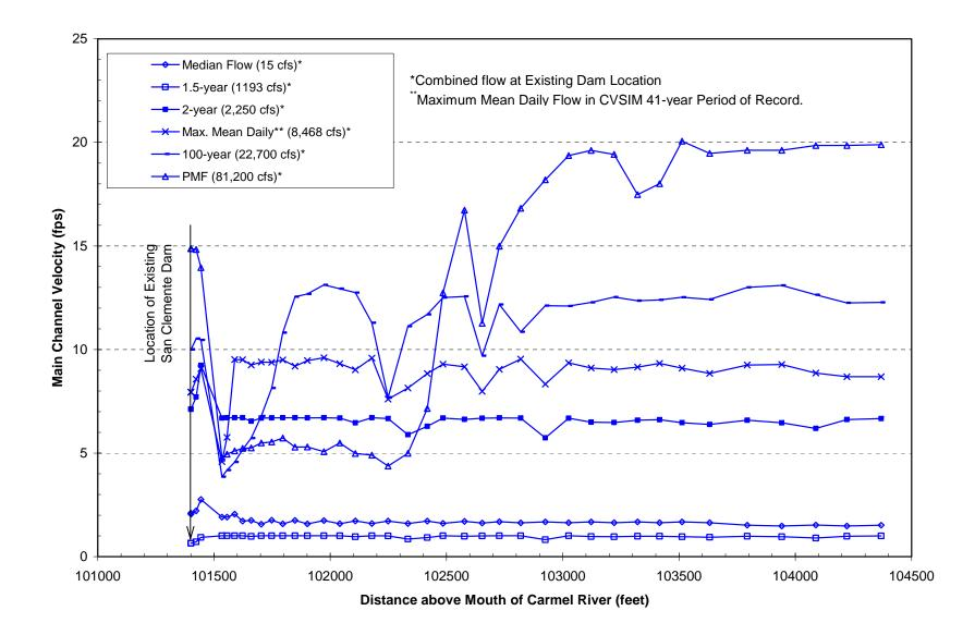
Figure 17. Computed main-channel velocity profiles for selected discharges in the San Clemente Creek Branch of San Clemente Reservoir under the Complete Dam Removal Alternative.
