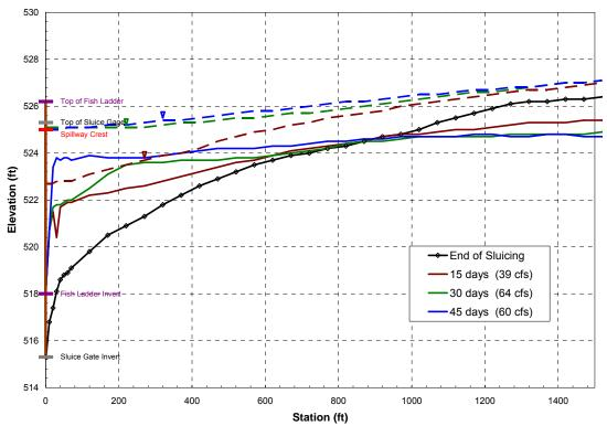
Figure 15b. Longitudinal profile of the incised channel upstream from the sluice gage at the end of the sluicing event, and 15, 30 and 45 days after the sluicing event, 1985 hydrology with fish ladder at full capacity.
