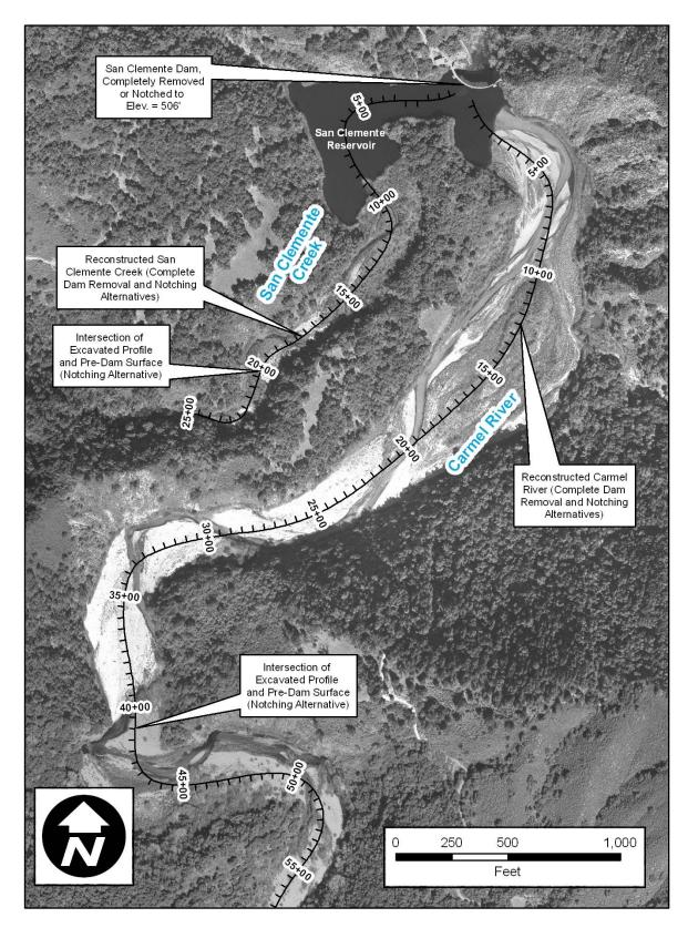
Figure 2. Proposed elements of the Complete Dam Removal and Dam Notching Alternatives.
