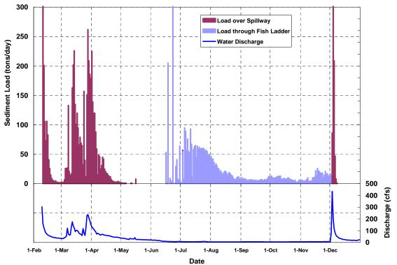
Figure 22. Sediment loads passing over the San Clemente Dam Spillway and through the fish ladder for the 1985 simulation. Also shown is the mean daily flow hydrograph for the simulation period (fish ladder discharge  $\leq 0$  cfs).
