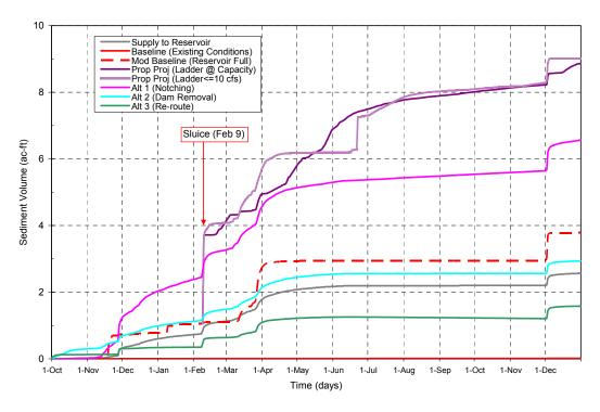
Figure 17. Cumulative sediment load passing San Clemente Dam from October 1, 1985, through December 31, 1985, for baseline and modified baseline (reservoir filled with sediment), Proponents Proposed Project, and Alternatives 1, 2 and 3).
