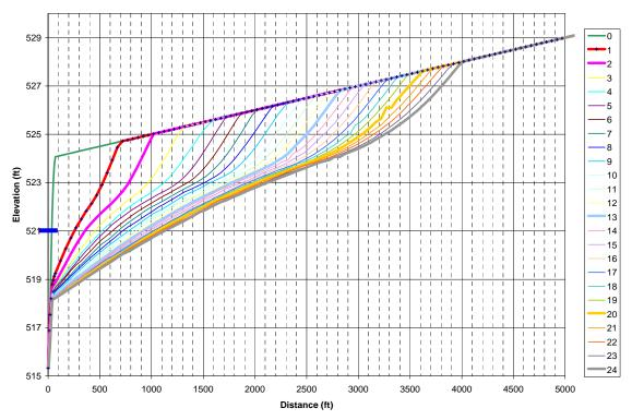
Figure 14. Estimated longitudinal profiles of the incised channel upstream from the sluice gate in 1-hour increments at a constant sluicing discharge of 300 cfs. Blue mark is water-surface elevation at sluice gate inlet.
