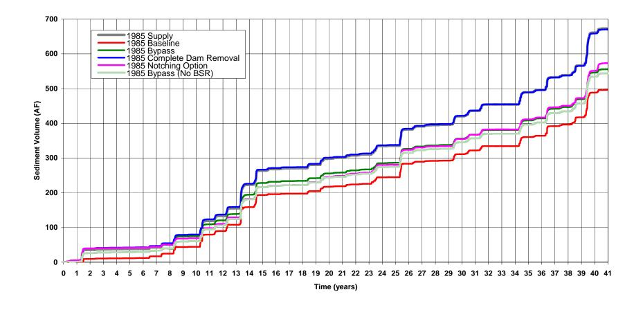
Figure 27. Inflowing base load and computed sediment load passing the location of the existing dam for baseline (with dam) conditions evaluated in MEI (2005) and for the Bypass, Complete Dam Removal, and Notching Alternatives evaluated in this study (1985 start date). Also shown are the results from the Bypass Alternative with no BSR evaluated in MEI (2005) for the 1985 start date.
