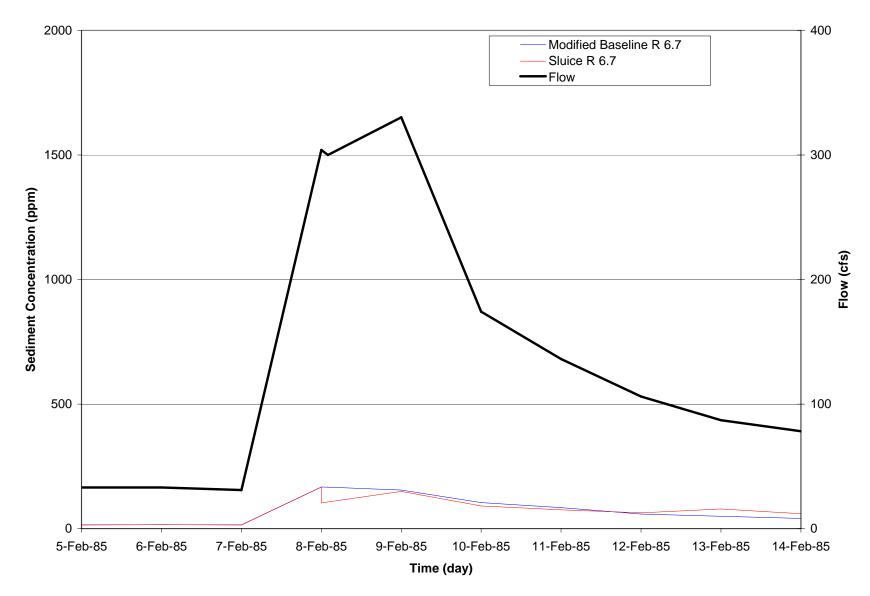
Figure O-19: Simulated Suspended Sediment Concentration at Reach 6.7 for a Dry Year
