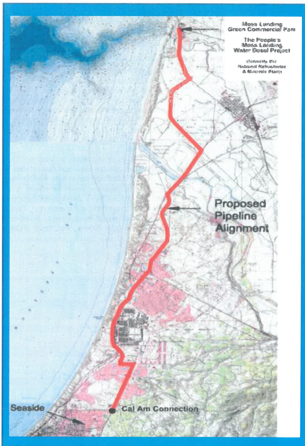
Figure 3 Proposed Transmission Pipeline
