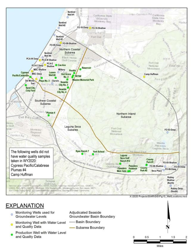
Figure 10. Wells Used for Seawater Intrusion Analyses
