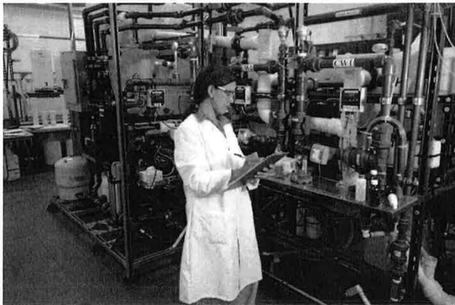
Figure 2 At the NSF residential water treatment system test facility, synthetic water challenges are produced for dosing of systems under test.
