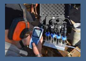
field parameters and collected for further lab analysis. The water quality monitoring is done as part of ASR permit requirements and to document how Carmel River water interacts with native Seaside groundwater.
