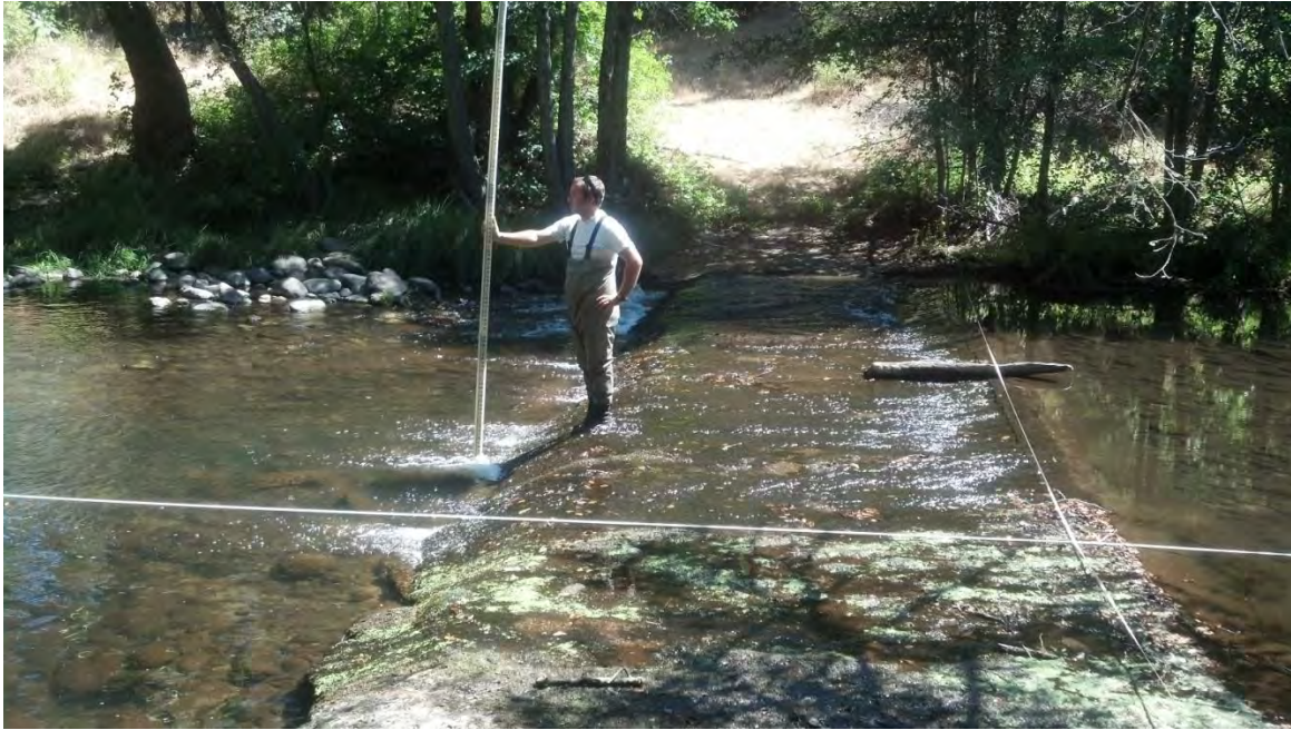
Photo 3) Looking across the ford from left bank. Note the shallow water depth across ford. Depth of plunge pool at this flow is ~1.5 feet.
