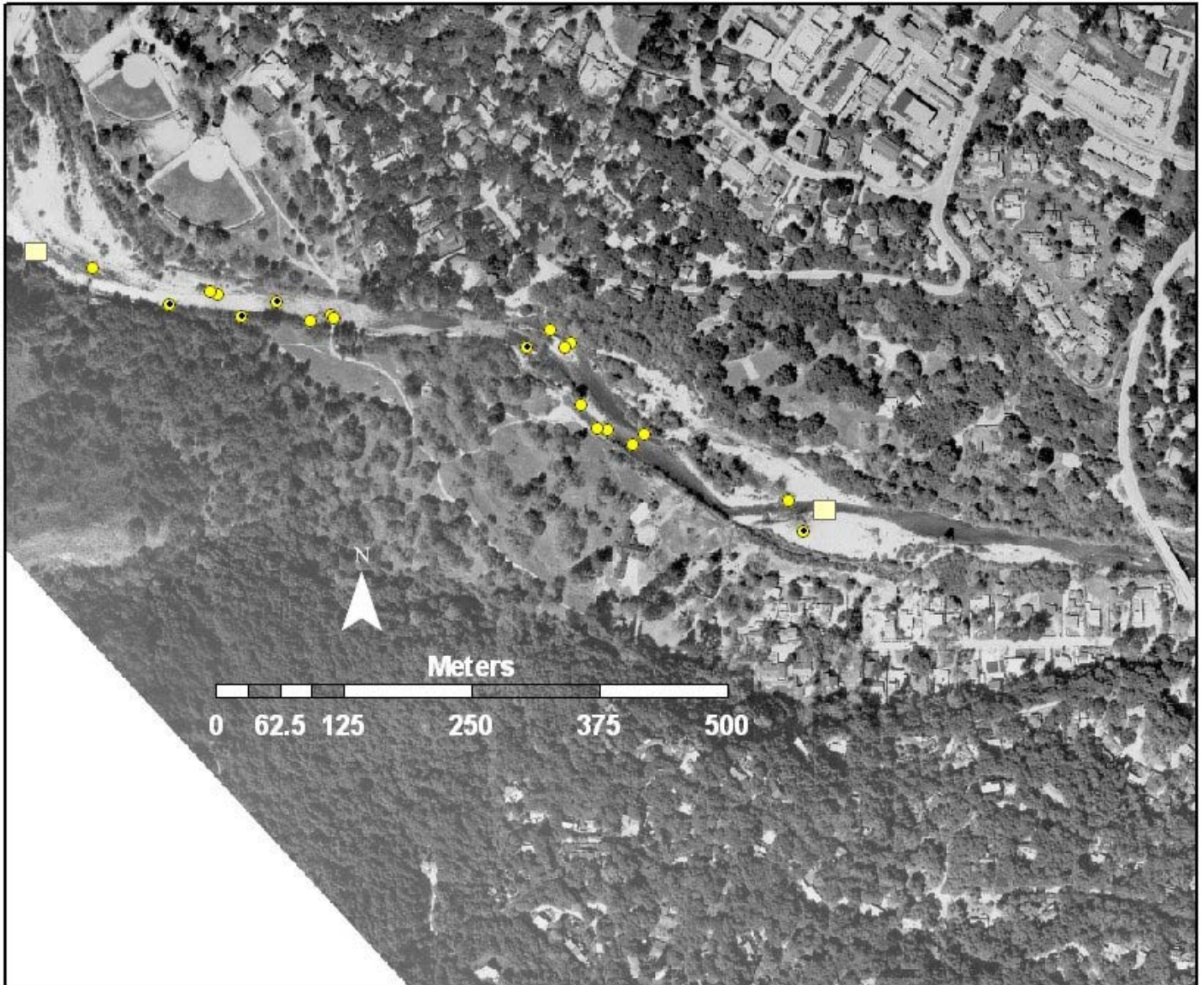
Figure 3: Details of LWD density between Rosies Bridge and deDampierre. Dots are single pieces of wood. Concentric dots are multiple pieces of wood. Boxes show the ends of the survey reach.
