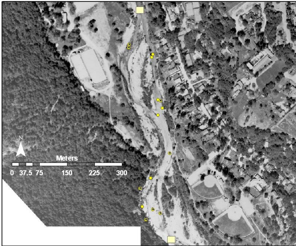
Figure 4: Details of LWD density along deDampierre. Dots are single pieces of wood. Concentric dots are multiple pieces of wood. Boxes show the ends of the survey reach.
