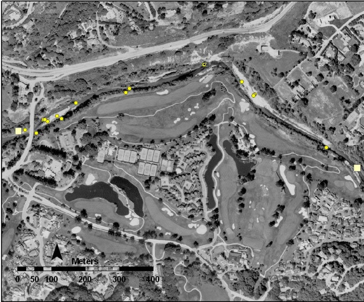
Figure 6: Details of LWD density between Scarlett Road and Robinson Canyon. Dots are single pieces of wood. Concentric dots are multiple pieces of wood. Boxes show the ends of the survey reach.
