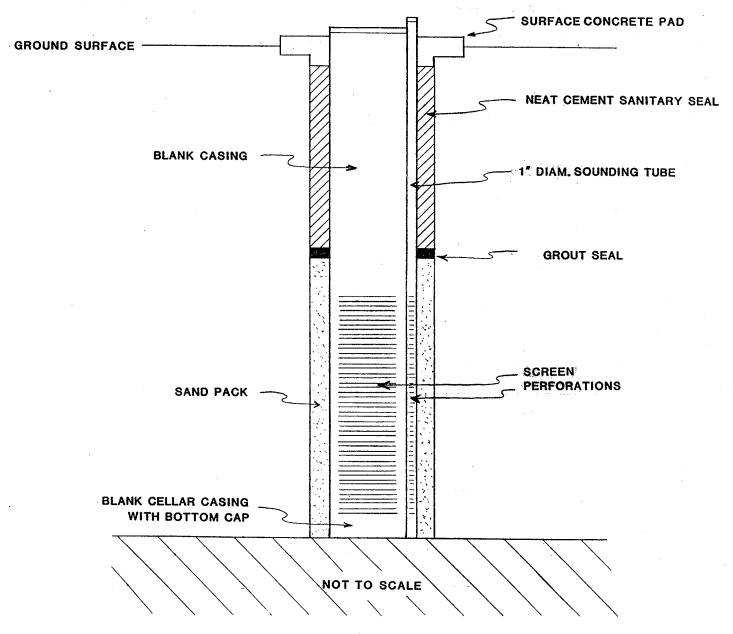
NOTE: ALL NEW WELLS WITHIN THE MONTEREY PENINSULA WATER MANAGEMENT DISTRICT MUST BE EQUIPPED WITH A SOUNDING TUBE. THE SKETCH SHOWN ABOVE ILLUSTRATES AN ACCEPTABLE METHOD FOR INSTALLING A SOUNDING TUBE. SOUNDING TUBE CAN BE STRAPPED TO OUTSIDE OF WELL CASING DURING INSTALLATION, OR MAY BE INSTALLED INSIDE WELL CASING. IN ANY EVENT, INSTALLATION SHOULD BE SUCH THAT A WATER LEVEL MONITORING DEVICE WILL NOT GET HUNG UP ON OTHER WELL PIPES, CABLES, ETC.
