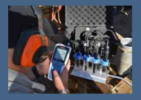
certian field parameters and collected for further lab analysis. The water quality monitoring is done as part ASR permit requirements and to document how Carmel River water interacts with native Seaside groundwater.
