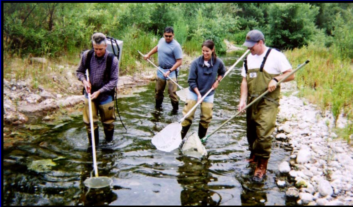
A backpack electrofisher and dip nets used to catch fish before the river dries up.
