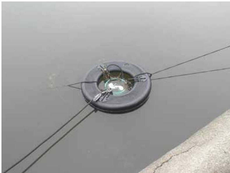
Figure 10.14 The second of two aeration machines installed in the South Arm of the Carmel Lagoon. Photo: Joel Casagrande, 14 Sep 03.
