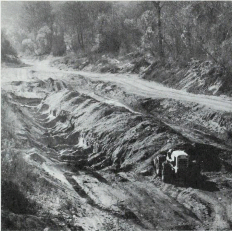
Photo 41. Valley Rock and Adobe Company's sand and gravel pit. This Carmel River stream channel deposit is narrow, being confined by levees over a distance of 15 miles upstream from the mouth. The stream normally flows most of the year, but after three successive "dry" winters the channel was completely dry in October 1961.
