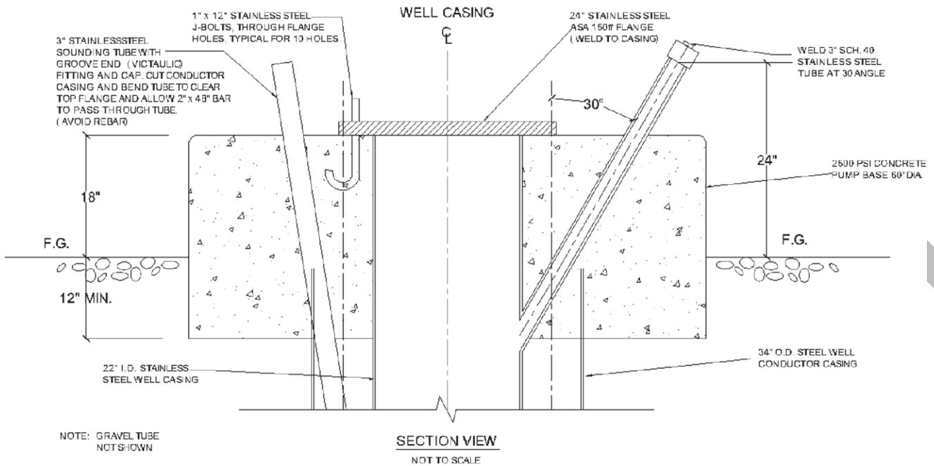
**FIGURE 5. WELLHEAD AND FOUNDATION DETAILS**
